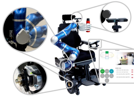
Figure 2.7: EDAN system including a closeup of the wheel-encoders, the 8-DOF robot, the head-switch, the RGB-D camera, and the tablet interface. Image reproduced as presented in [7].
