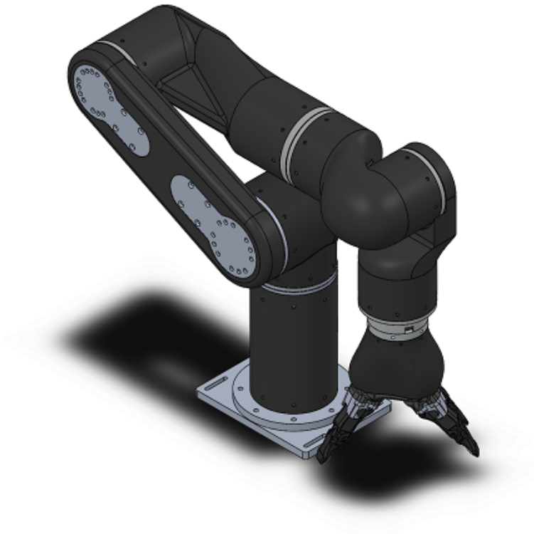
Figure 5.8: CAD Model Illustrating the Folded State of the Optimal Assistive Robot
