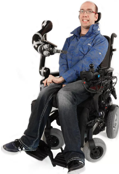
Figure 2.4: JACO mounted on a power wheelchair. Image reproduced from [4]
