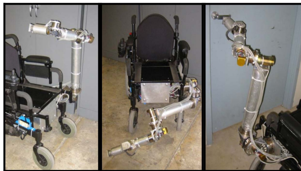
Figure 2.6: WMRA in a feeding pose, low-right reach, left side doorknob. Image reproduced from [6]
