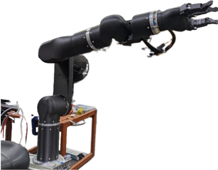
Figure 5.6: Optimized Assistive Robot: This figure illustrates the final design of the assistive robot with link lengths derived from the optimization process. The optimized design aims for maximum workspace while minimizing energy consumption.
