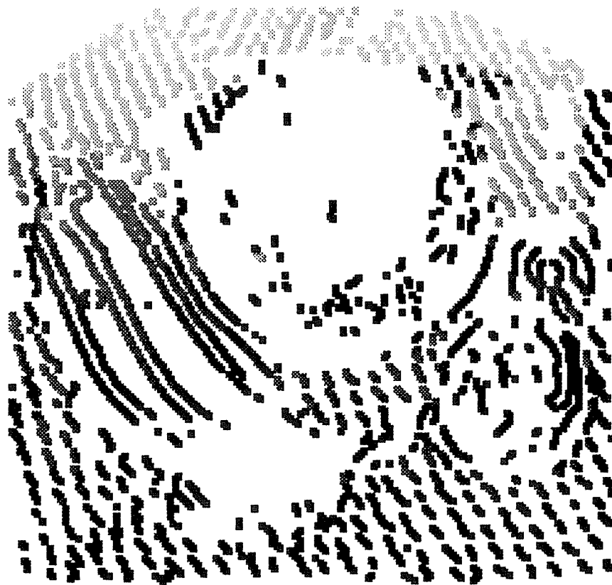
(c) Level 1 disparity image resulting from matching. Non-white pixels are expanded into a 3 by 3 neighborhood.
