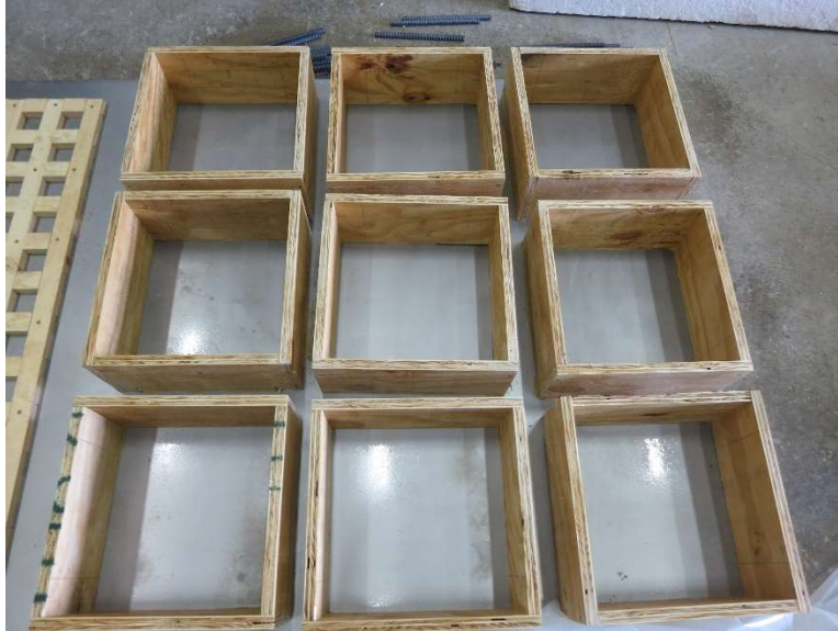
Figure 4-1: Typical concrete sample formwork.
