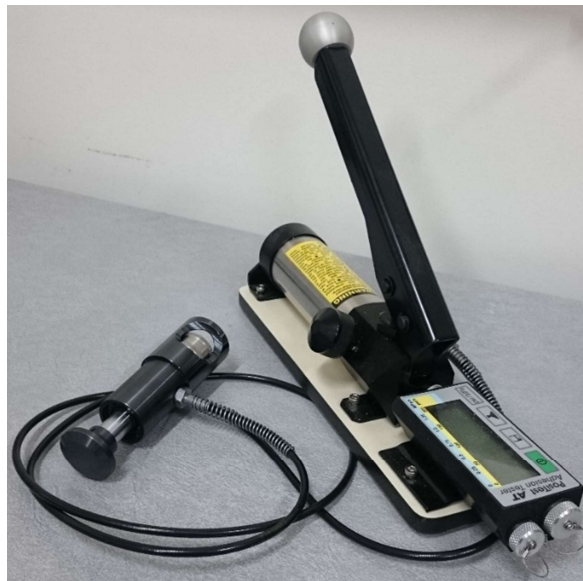
Figure 4-18: Manual pull-off adhesion tester.
