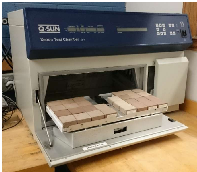
Figure 4-13: Xenon Arc test chamber, with an uninsulated black panel for temperature measurement.
