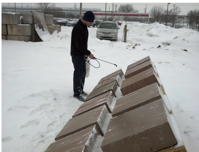
Figure 4-21: Outdoor weathering exposure rack and saline solution application procedure.
