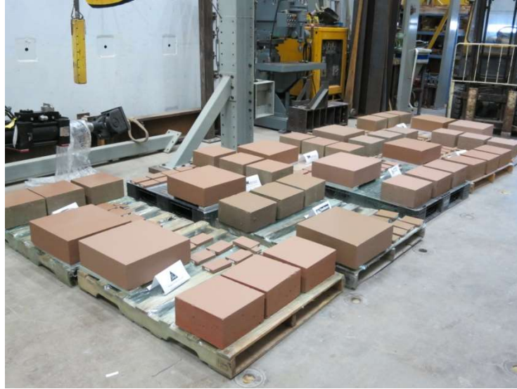
Figure 4-6: Sample curing conditions following coating application.
