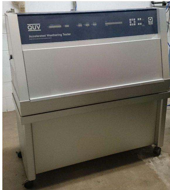
Figure 4-9: UV/Condensation accelerated weathering chamber.
