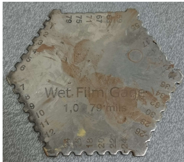
Figure 4-5: Wet film gage used during coating application.
