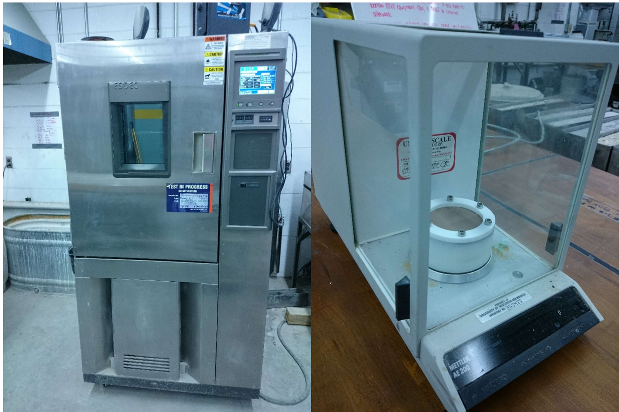
Figure 4-23: Environmental chamber (Right) and scale (Left) used for the evaluations of water vapor transmission.
