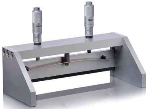
Figure 4-22: Adjustable film casting knife (Left) and a prepared permeability dish with test specimen (Right).
