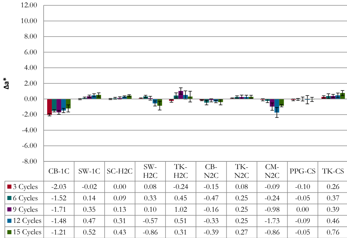
Figure 5-3 UV/Prohesion mean \Delta a^* values throughout exposure period with 95% confidence intervals.
