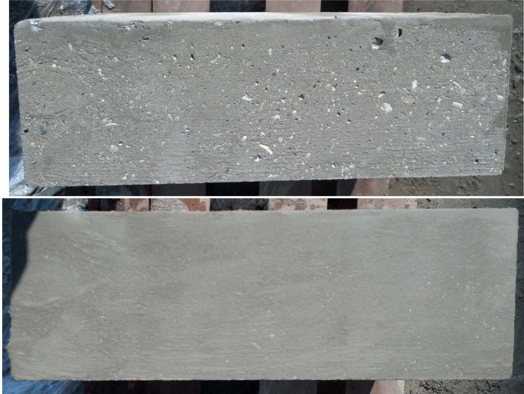
Figure 4-3: Concrete specimen before and after sack rubbing surface treatment.
