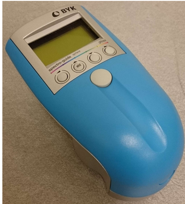
Figure 4-15: Spectrophotometer used for color and gloss evaluations.
