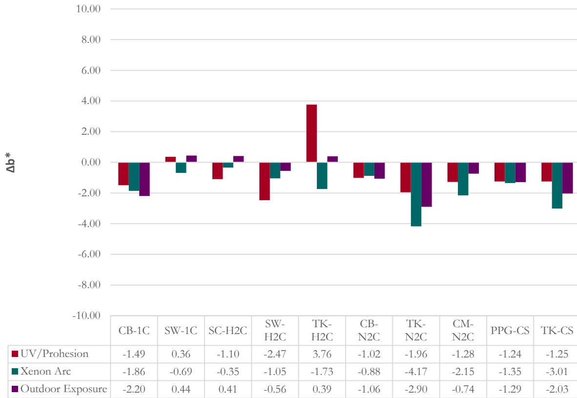
Figure 5-22: Maximum recorded \Delta b^* from each weathering exposure by coating system.
