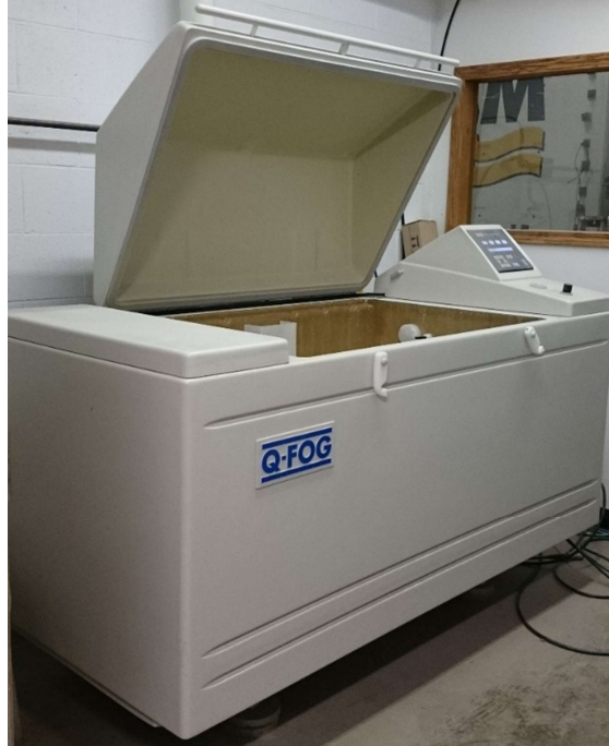
Figure 4-10: Cyclic salt fog corrosion testing chamber.
