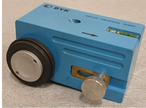
Figure 4-17: Pencil hardness tester.
