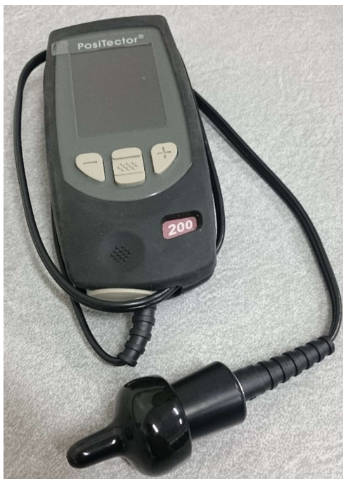
Figure 4-16: Ultrasonic coating thickness gage used to determine dry film thickness.
