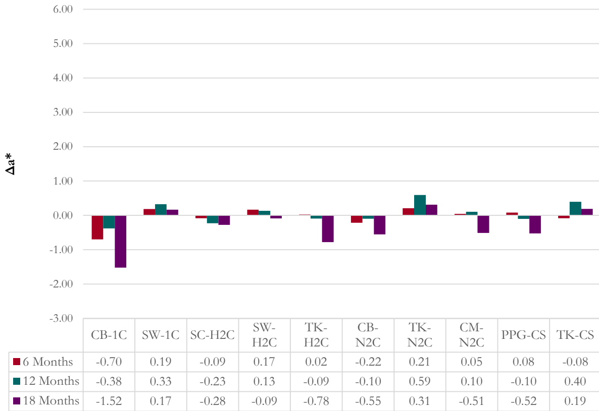
Figure 5-16: Average \Delta a^* values of each coating system throughout outdoor exposure.
