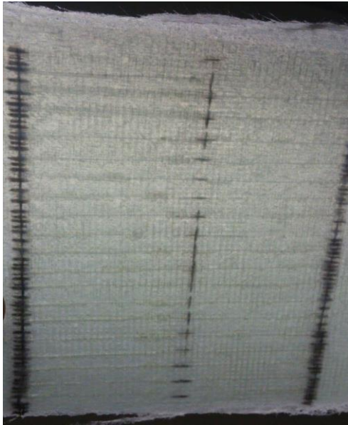
Figure 14. Fiberglass reinforced polymer composite with a central layer of hollow Borosilicate tubes
