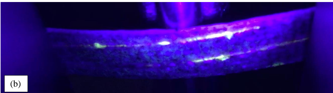
Figure 46: Photographs (a) and (b) of a specimen from sample 9 during three-point bending test showing evident signs of filling of cracks by the healing agent (glowing liquid). Image (a) is at the start of the test and (b) is to the end of the test. Specimen is S9B2
