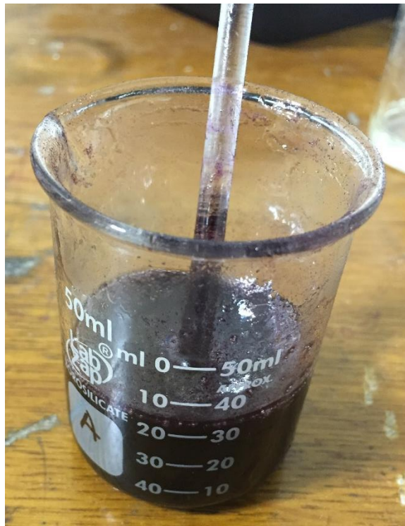
Figure 94: Concentrated Grubb's catalyst mixture used specifically around the tubes
