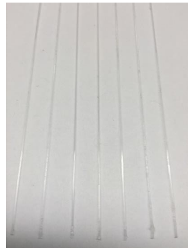
Figure 15. 500µm outer diameter Borosilicate tubes filled with Dicyclopentadiene/healing agent
