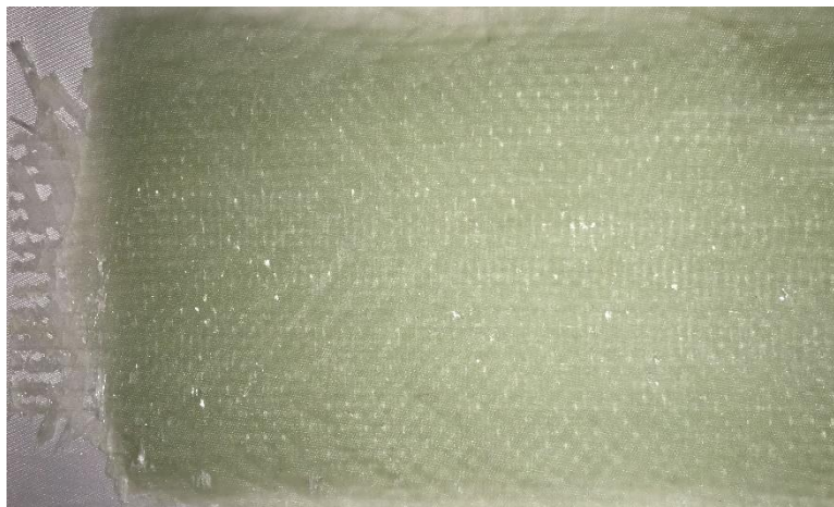
Figure 9: Photograph of the mold with a layer of PVA strings as central layer
