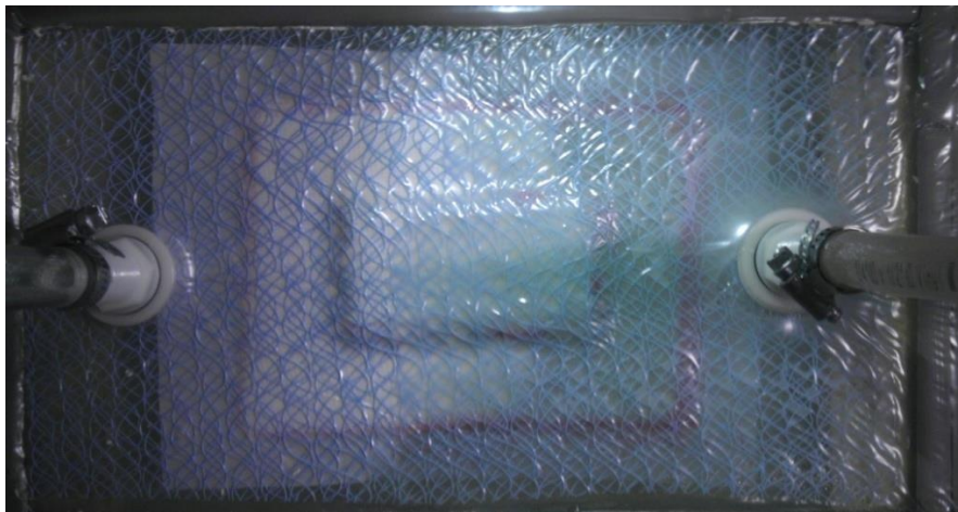
Figure 5. Photograph during the molding process of sample D. Resin-hardener mixture is flowing from right to left. A similar process was used for the preparation of the mold used to obtain sample “E,” the only difference being the orientation of microtubes.
