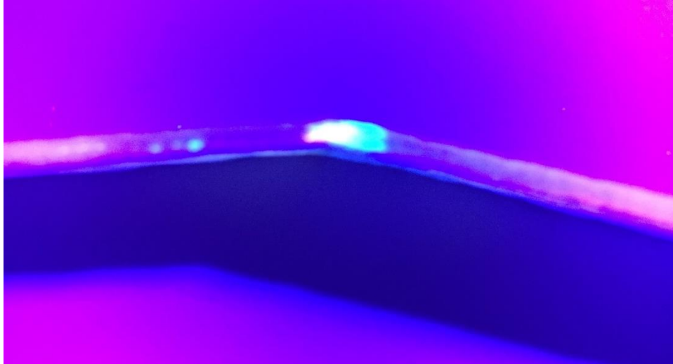
Figure 38: Photograph of a side of one of the specimens from sample 3 showing bleeding of tubes along the line of flexural load
