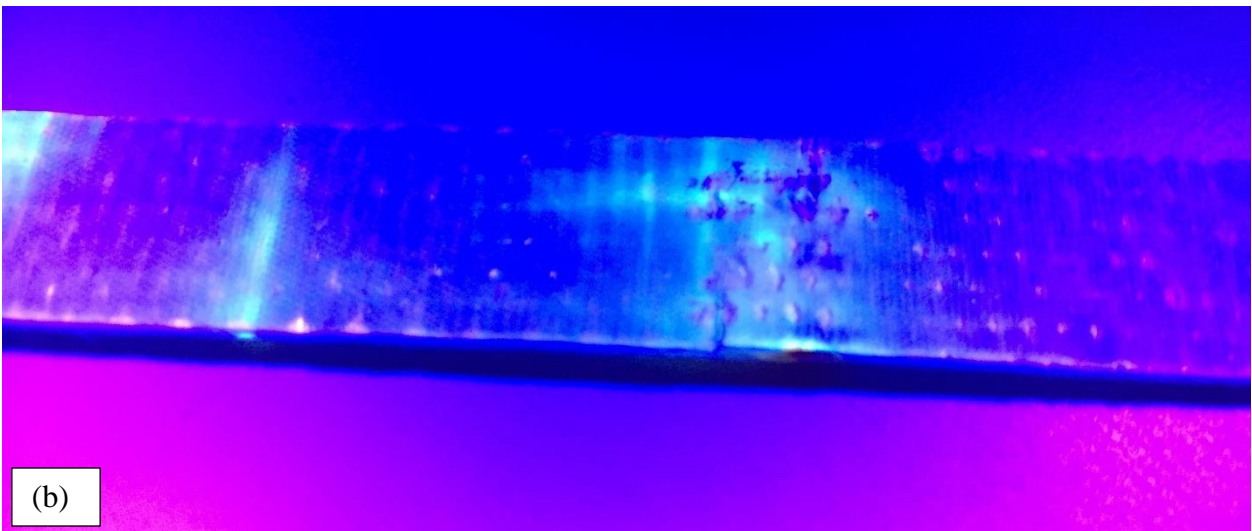
Figure 33: Photographs of two specimens are shown in (a) and (b) after completion of tensile testing of the two specimens' with-tubes showing bleeding of healing agent (glowing liquid) at their damage locations
