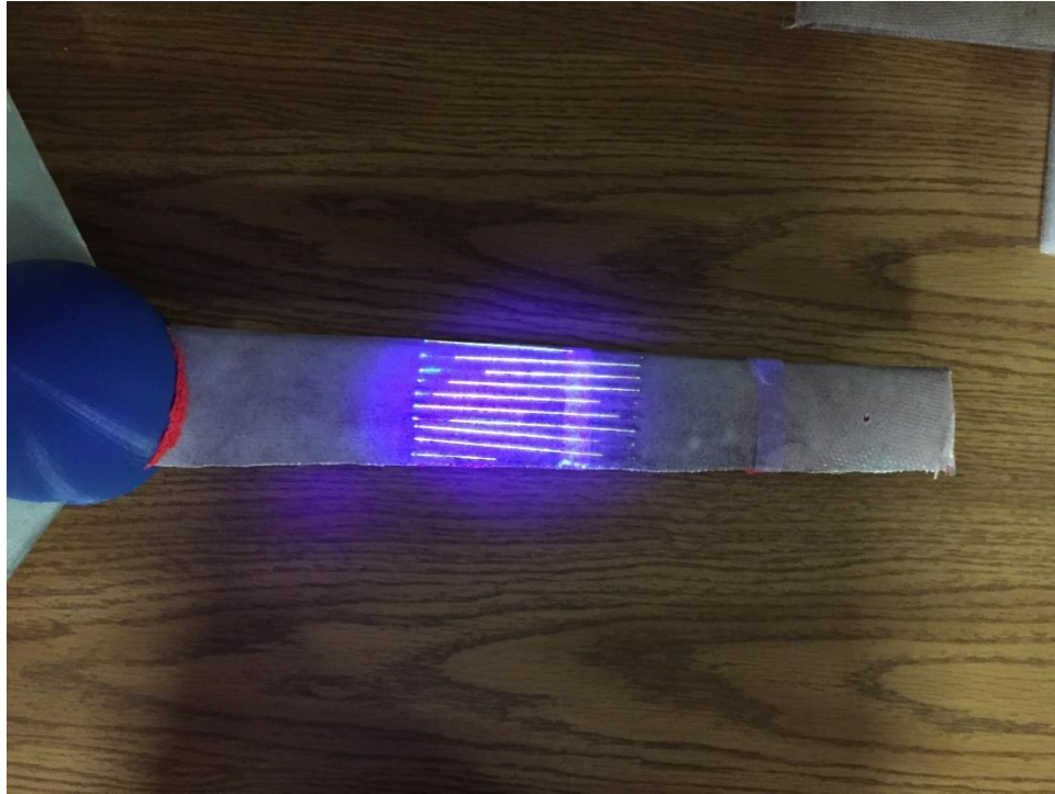
Figure 69: Photograph of a blade with self-healing characteristic fixed to scaled down wind turbine
