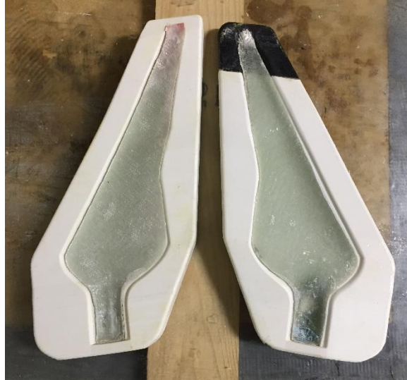
Figure 56: Photograph of both sides of molded pieces of wind turbine blade inside the 3D printed molds The vacuum pump was left running until the mold was cured to the leakage in a vacuum bag. Figure 57 and Figure 58 show the molded part that had dry spots due to the intricate shape of the mold.
