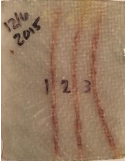
Figure 10: Photograph of PVA strings with sugar syrup coat (red dye used to check hollowness)
