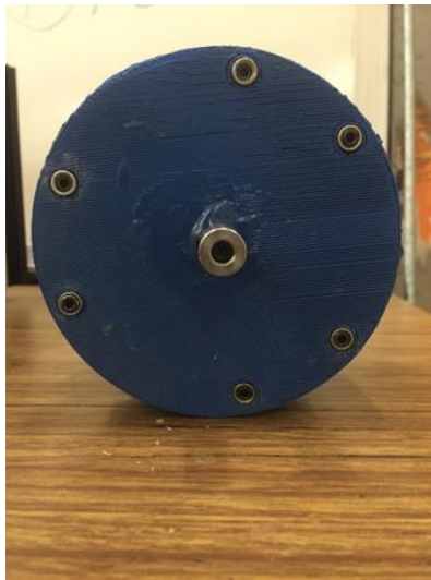
Figure 63: Photograph showing the back view of the 3D printed hub with the set screw location
