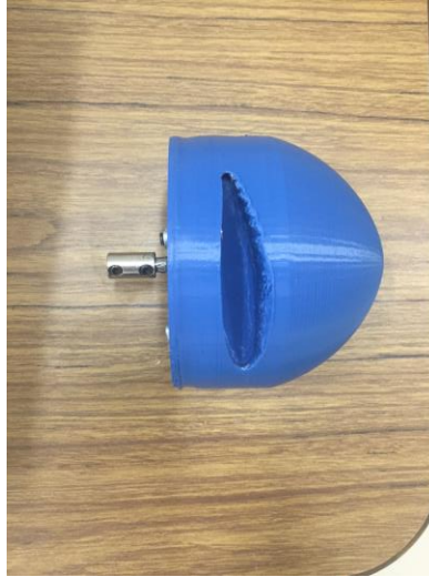
Figure 64: Side view of the 3D printed hub. View shows the groove for the blade and the coupling used to connect to the motor shaft
