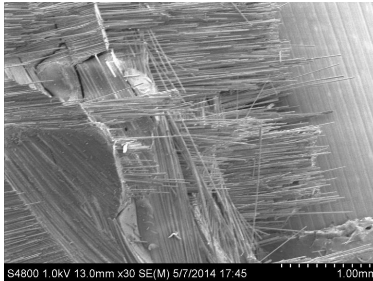
Figure 22. Scanning Electron Microscope image of the fracture surface of the composite with uniform fiber orientation between layers and molded by VARTM process (Sample II)
