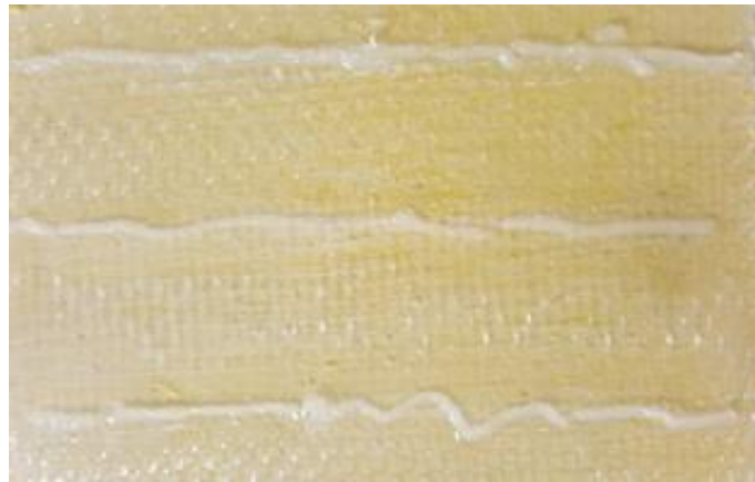
Figure 11: Distribution of the mixture proved difficult due to the high viscosity of the material
