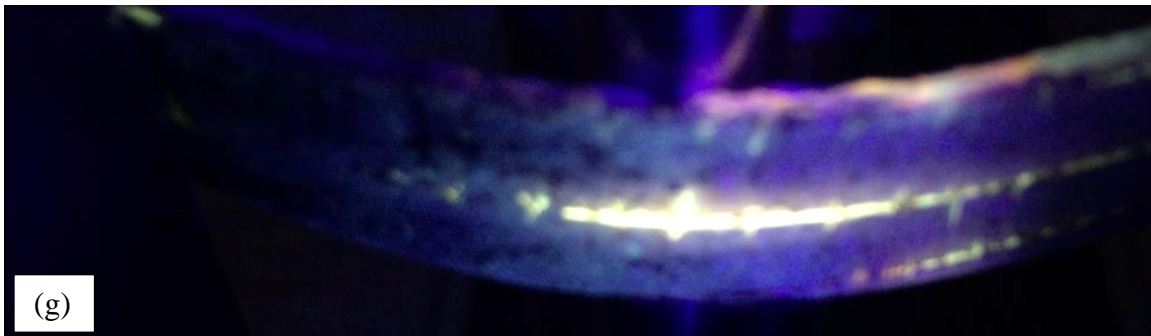
Figure 41: Photographs (a) to (g) of a specimen during three-point bending test showing evident signs of breakage, bleeding of the tubes and spreading of healing agent (glowing liquid) through the thickness of the composite. (a) being earliest and (g) being latest photograph. Image (a) is at the start of the test and (b) through (g) have 15s interval between the images to the end of the test (Specimen is S7B4)
