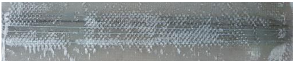
Figure 6: Photograph of the as-molded sample with floral stem wires embedded in it.
