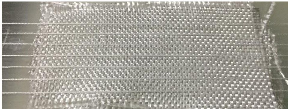
Figure 8: Arrangement of the PVA threads in the middle of fiber glass layers. The threads were glued to the vacuum tape to retain its shape
