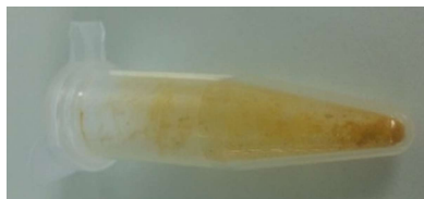
Figure 5-13 Reformed lead iodide for solar cells from waste lead solids.
