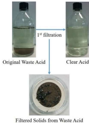
Figure 5-4 Raw waste acid pretreatment. Original waste acid was filtrated for later metal ion separation. Filtered solids were introduced to lead material refinement.
