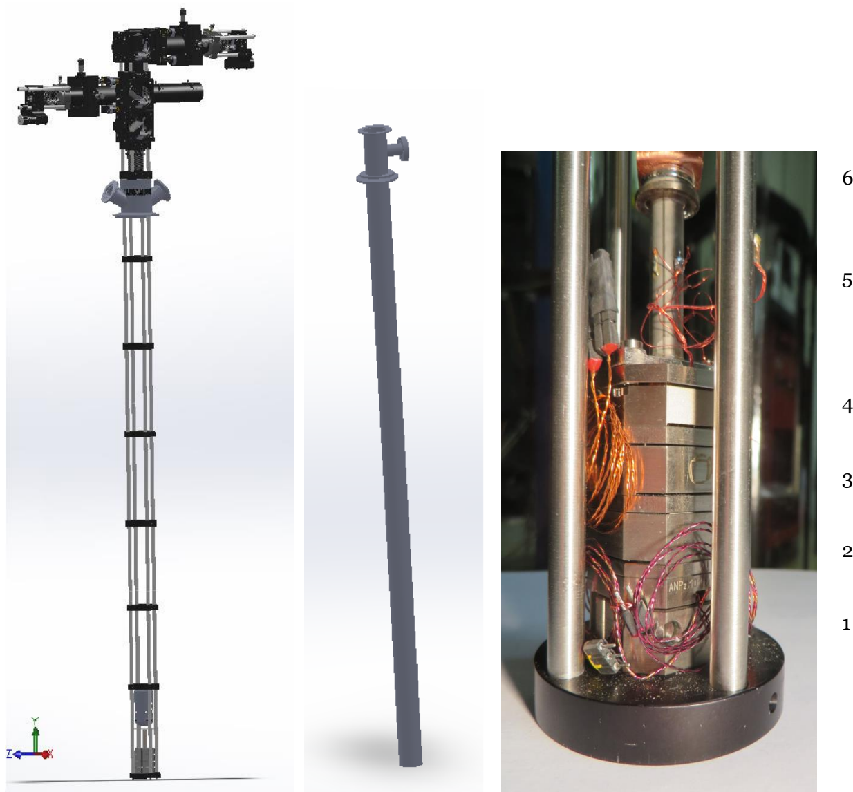
Figure 4.6: Left: The complete CTCSM, microscope head and the optical insert. Samples sit below the objective atop the positioners at the base of the optical insert portion of the CTCSM. Center: Insert tube that houses the optical insert when the microscope is used within the cryostat. Right: Close-up of the sample stage and piezo actuators used for coarse positioning and the raster process. Components as numbered 6. sample stage, 5. PI PT 130.14 piezo tube (raster scan), 4. ANSxy100lr (new raster scan positioner), 3. ANPx101 (X direction), 2. ANPx101 (Y direction), 1. ANPz101 (Z direction).
