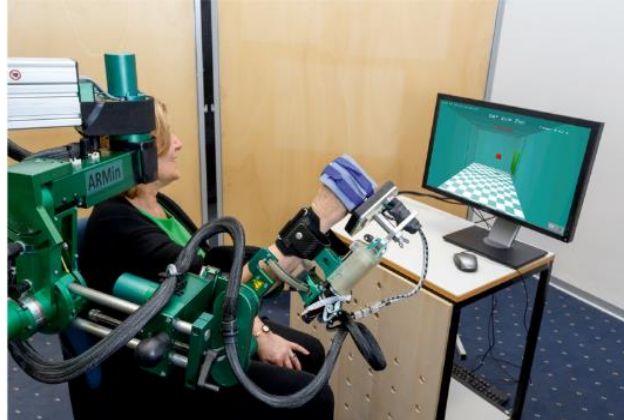
Figure 2.1 ARMin-III robot in use [12]
