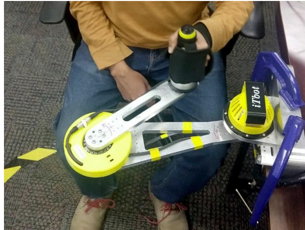
Figure 6.9 Horizontal Configuration of iTbot
