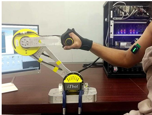
Figure 7.2 Active exercise with EMG data acquisition
