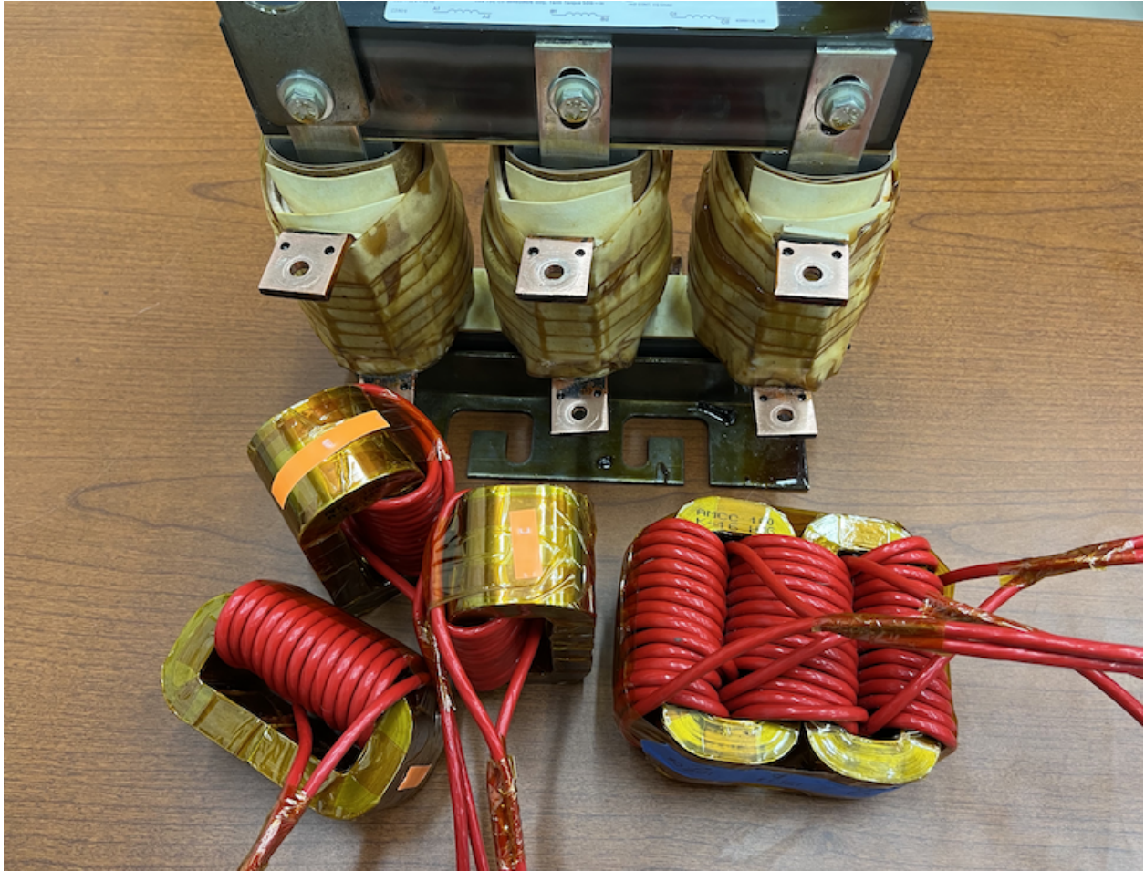
Figure 4.16: Inductors used in this study (Upper: TCI V1K130A00; Lower-left: Custom-made separate-cores; Lower-right: Custom-made common-core.)
