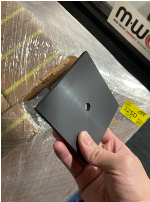
(a) Ferrite tile used in chamber
