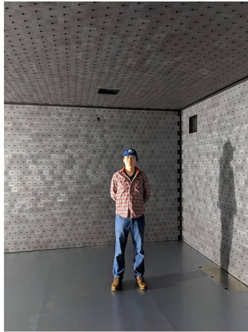
(b) Author standing in the chamber with absorbers visible on interior walls and ceiling
