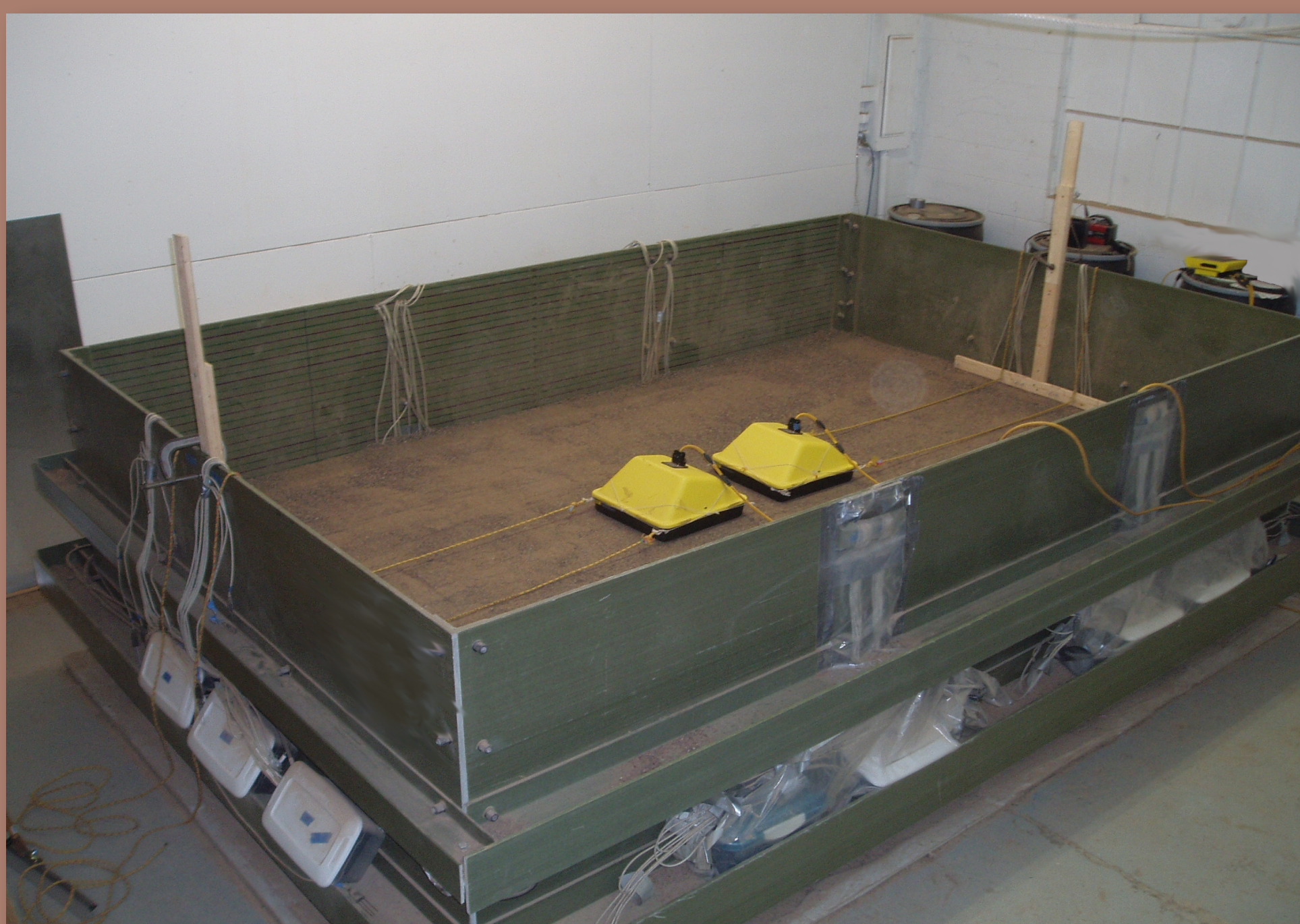
Figure 2: Common-midpoint surveys were performed in the middle of the tank for each GPR frequency. To avoid compaction of the soil, no one entered the tank after soil was added. The antennas were moved remotely using ropes.
