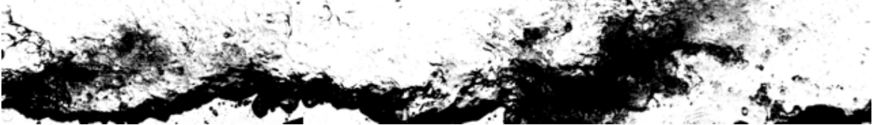
Figure 5-5 Normal water surface tension (0.074N/m) with V_{air}=40m/s (Time interval = 10 msec)
