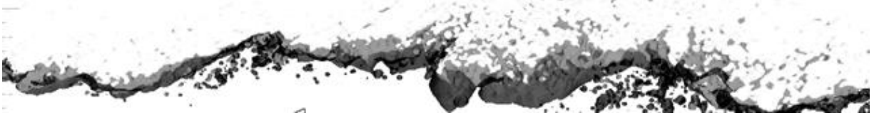
Figure 6-11 Normal water surface tension simulation (0.074N/m) with V_{air}=30m/s (Time interval = 10 msec)
