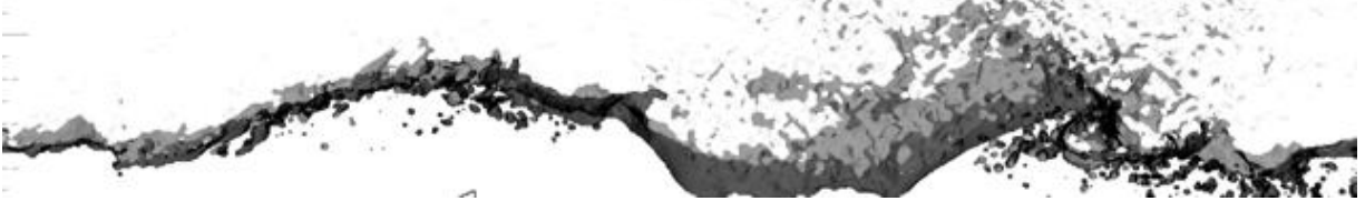
Figure 6-12 Reduced water surface tension Simulation (0.040N/m) with V_{air}=30m/s (Time interval = 10 msec)
