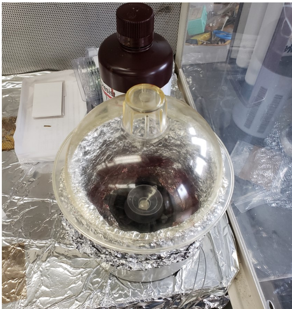
FIGURE 3.13: Home built spin coater used for the fabrication of large-array nanoparticle devices.
