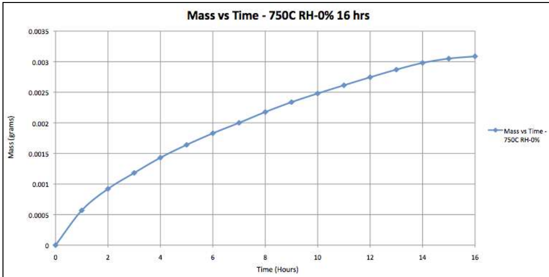
Figure 13. Time vs. Mass, isothermal at 750°C and 0% of Relative Humidity during 16 hours.
