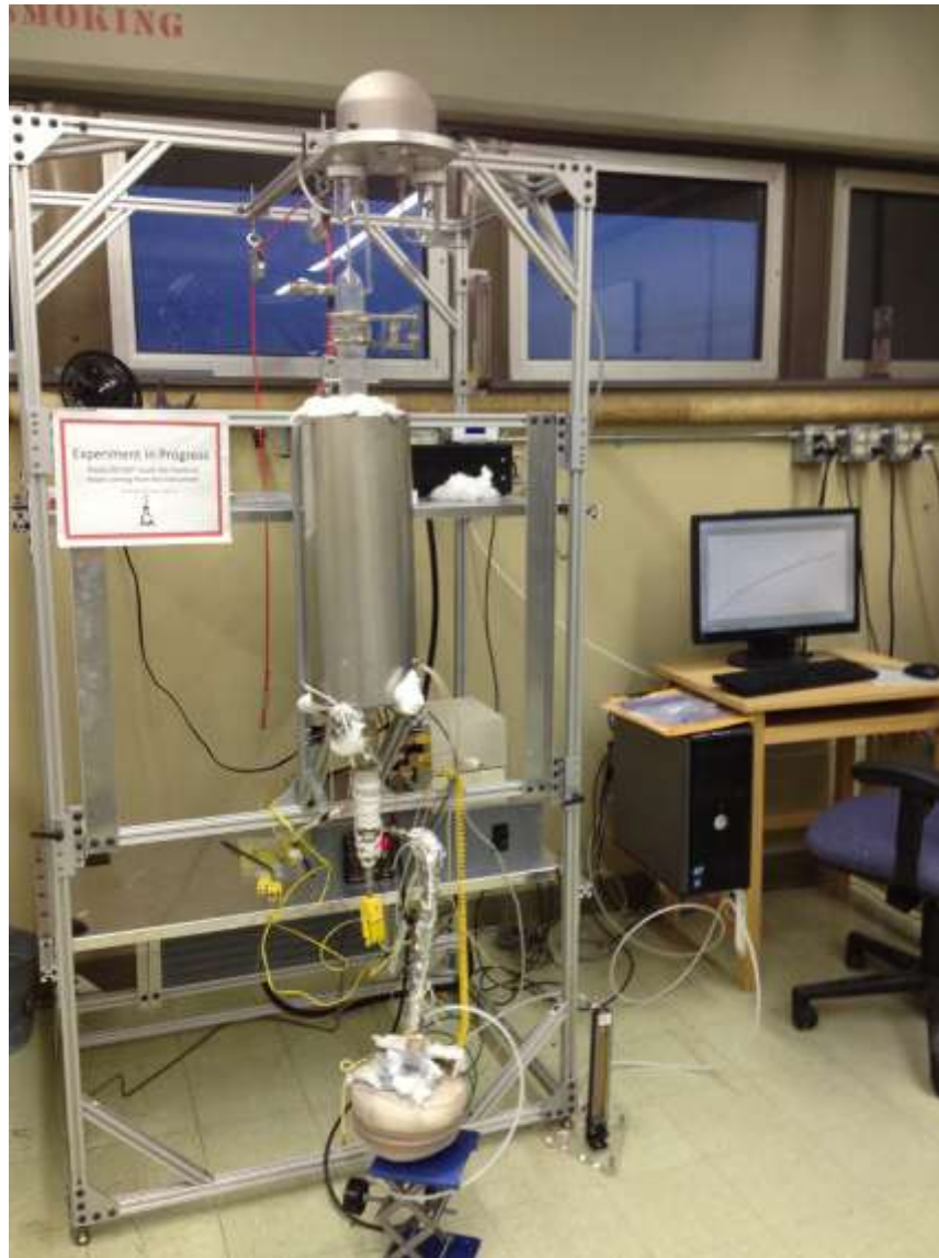
Figure 12. Custom built Thermogravimetric Analysis Equipment
