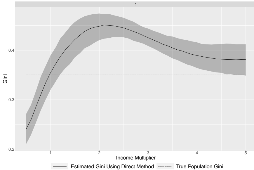
Figure 1.45: Performance of “Direct Method” for Estimation of the Gini Index, with Finer Bin Structure Gini estimated using the “Direct Method” on binned data created by random sampling from a population with a lognormal distribution of incomes with a location parameter of 3.5 and a scale parameter varying from 1-1.3. Samples then scaled from one half to five times their original value. Line is median estimate, bands represent the central 90% of estimates from random sampling from the distribution. Using finer bin structure.
