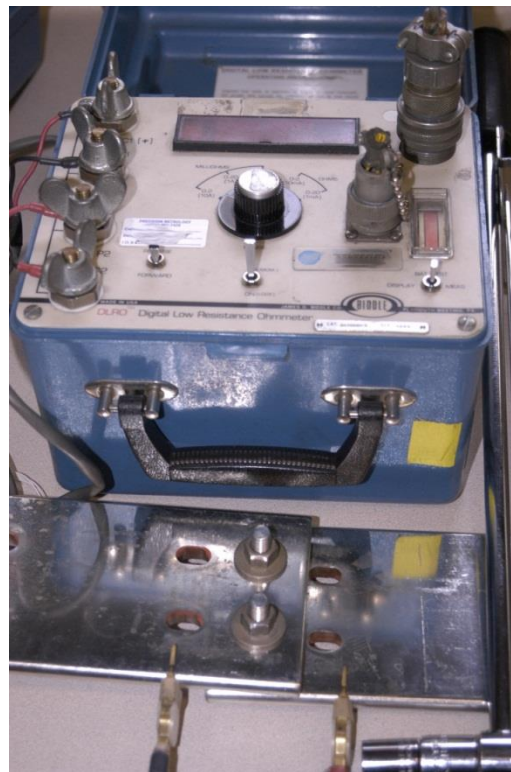
Figure 3-2. Resistance Measurement Experiment Set-Up.
