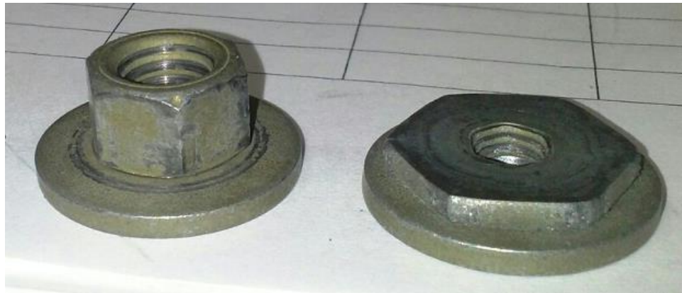
Figure 2-12. Before and After Comparison of Compressed Nut Sample.
