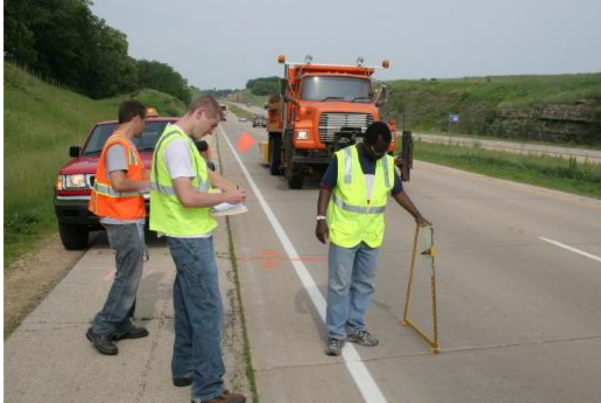
Figure 4.1 Transverse Joint Fault Measurement on USH 18/151
