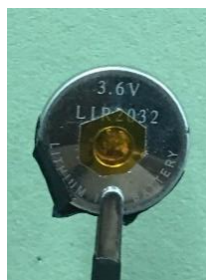
Figure 47. Nano-battery for the TXM test.
