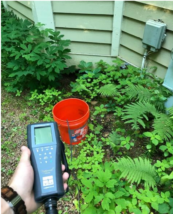
Figure 23. Measuring field parameters using YSI Professional Plus multiparameter instrument at location L3.
