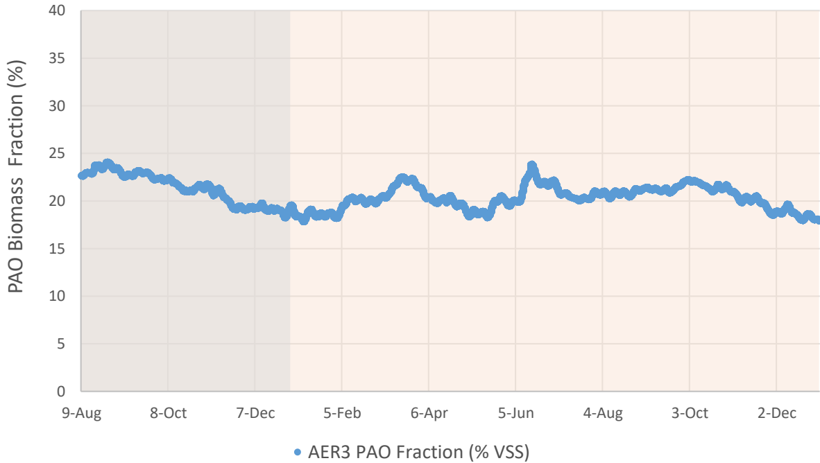
Figure 4.19 Variable DO model simulation PAO population fraction of biomass (% VSS) (08/09/2016 to 12/31/2017; shaded regions delineate year)
