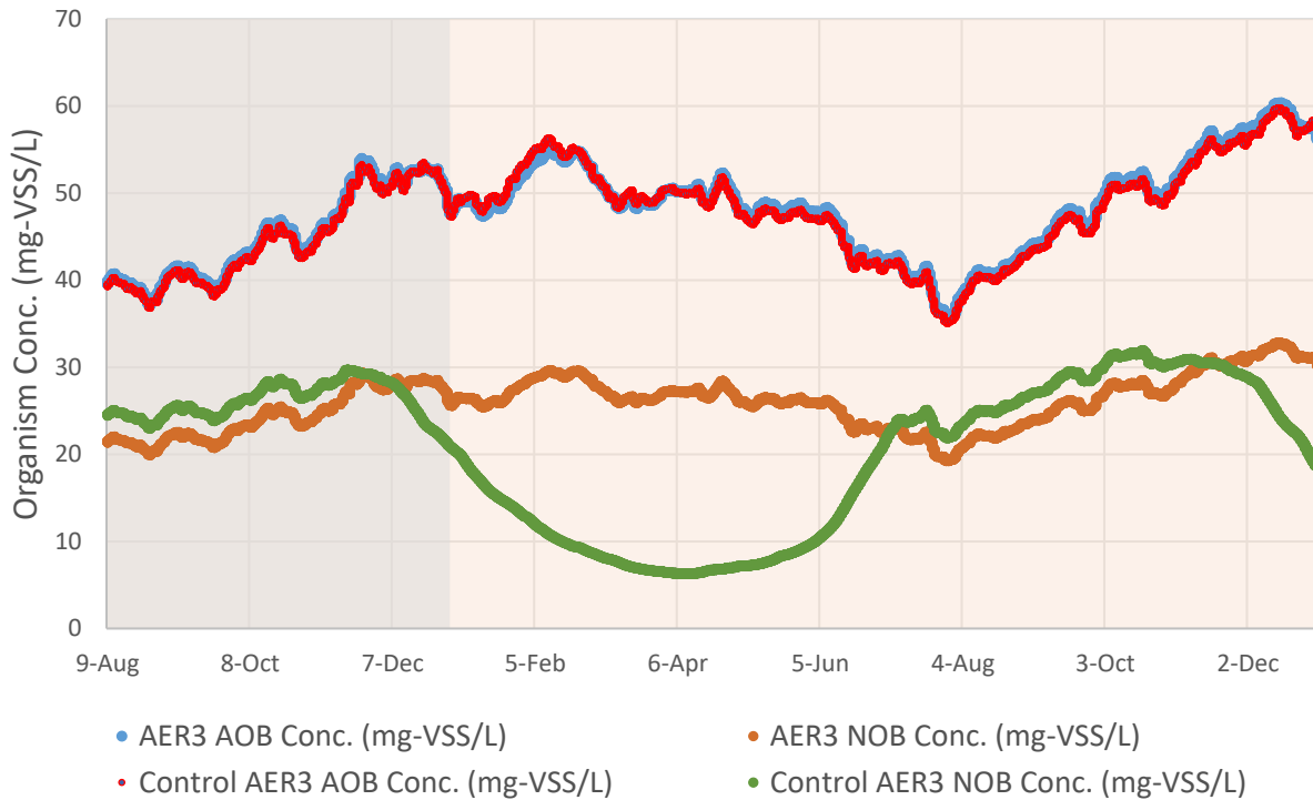
Figure 4.9 Kinetic model simulation compared to control simulation AOB and NOB population (08/09/2016 to 12/31/2017; shaded regions delineate year)
