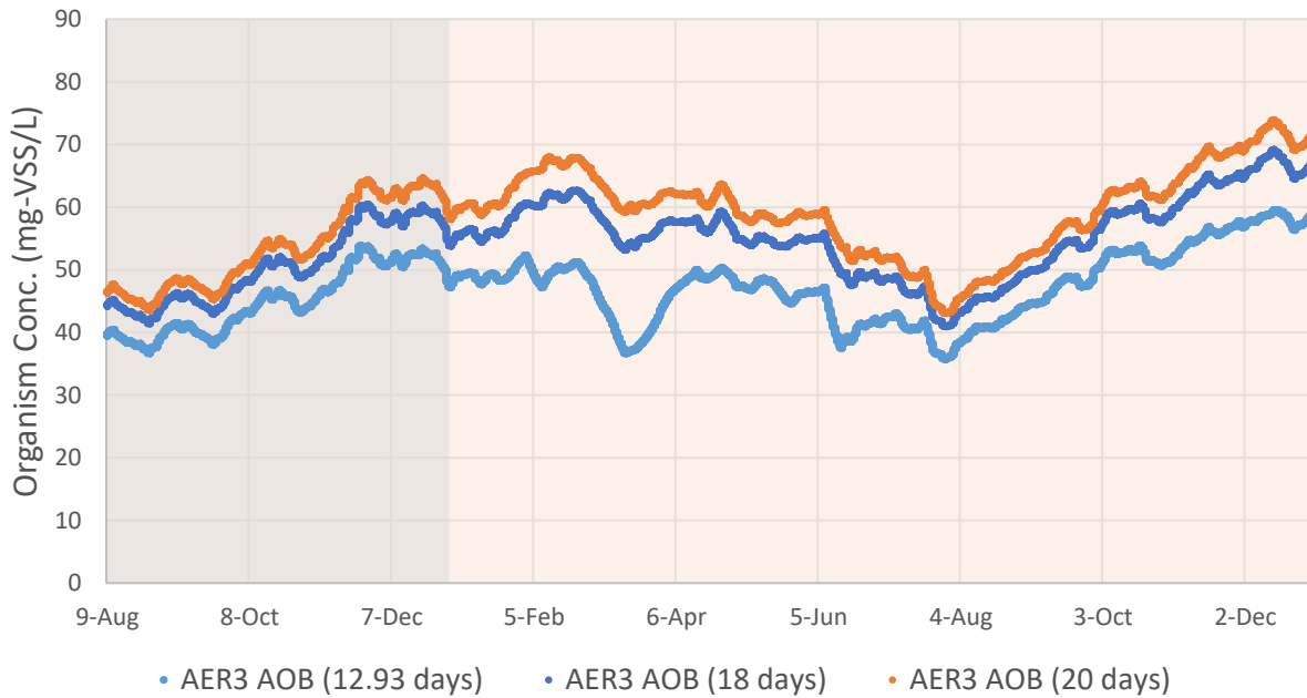
Figure 5.2 AOB concentration for SRT increase to 18 and 20 days (08/09/2016 to 12/31/2017; shaded regions delineate year)
