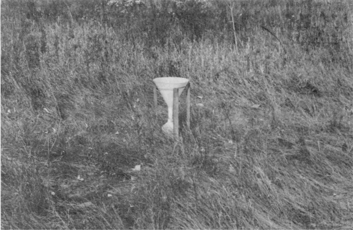
Figure 2. Rainfall collector located in open field.
