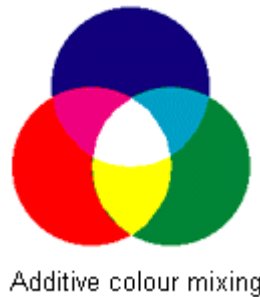
Figure 5.1: Additive color mixing using red, green, and blue primaries (Finbury, 2004)
