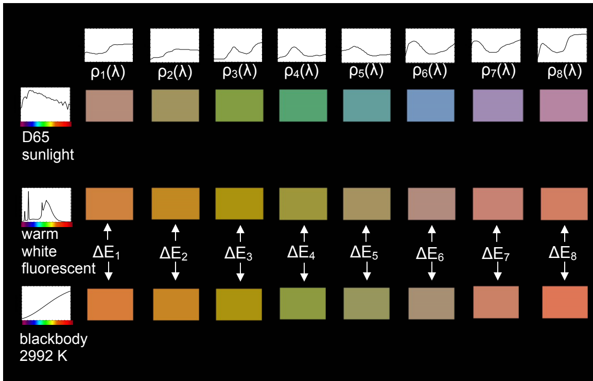
Figure 5.20: The color of the eight color samples, \rho(\lambda) , illuminated in turn by D65, the warm white fluorescent lamp described in Chapter 4, and a 2992 K blackbody spectrum. \Delta E indicates the color difference for a given color sample between two illuminants.
