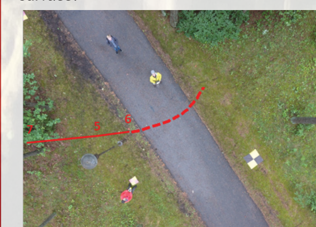
Figure 4: Aerial imagery of showing the high resistance locations from ERT results (7, 5, and 6). Dashed line indicates the hypothetical path of the tunnel (WorleyParsons 2016)
