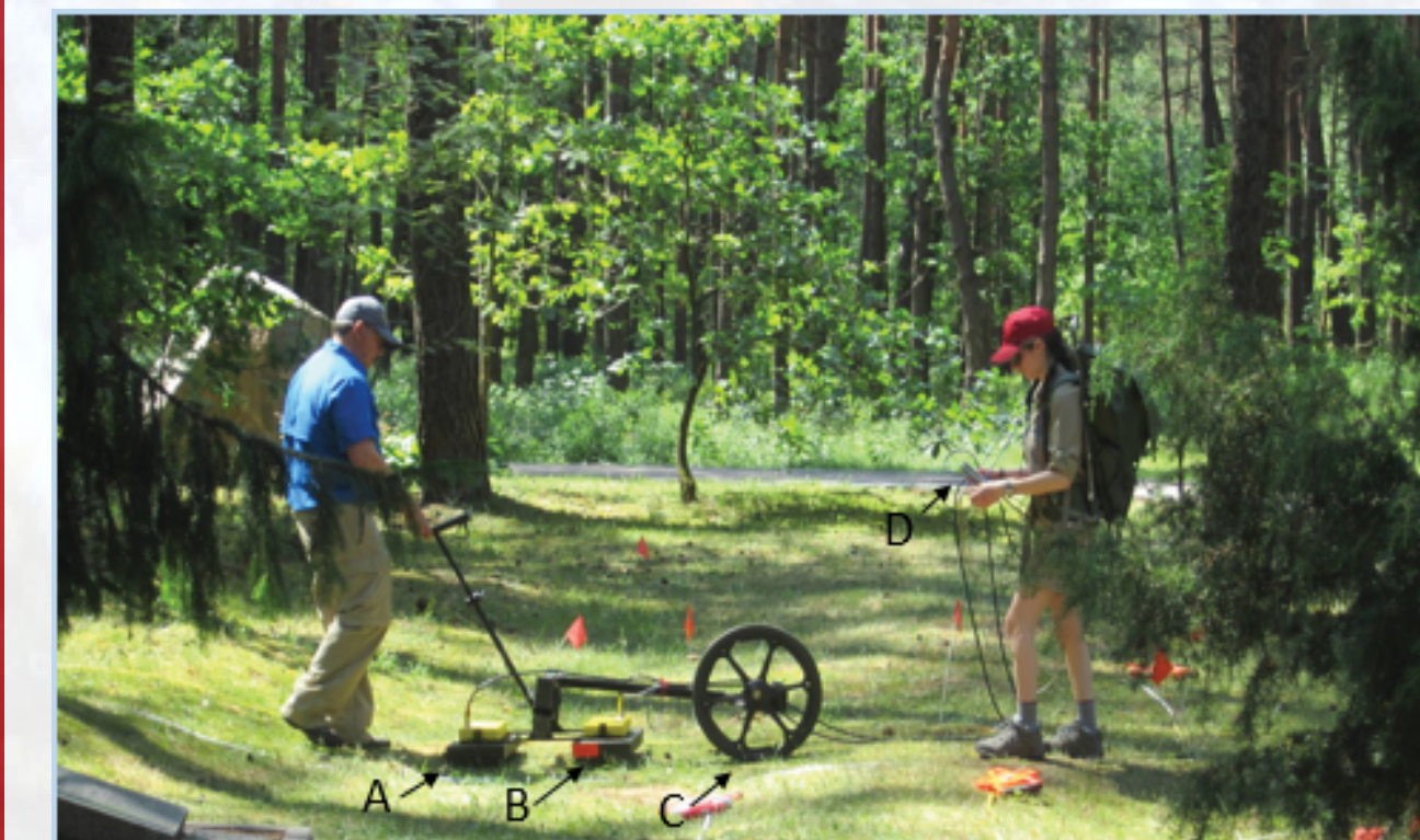
Figure 8: Sensors and Software pulseEKKO1000 consisting of A) Transmitting antenna, B) Receiving antenna, C) wheel with odometer, and D) Computer that records data in real-time (Erickson 2016)
