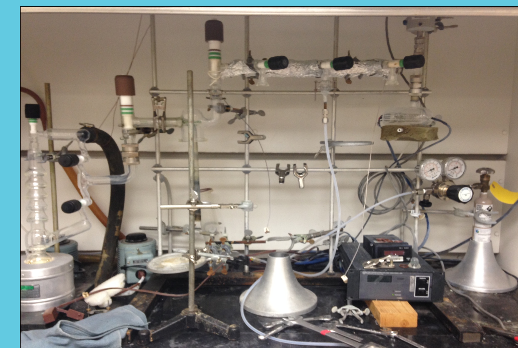
Above: Manifold, where gas mixtures are made under vacuum
