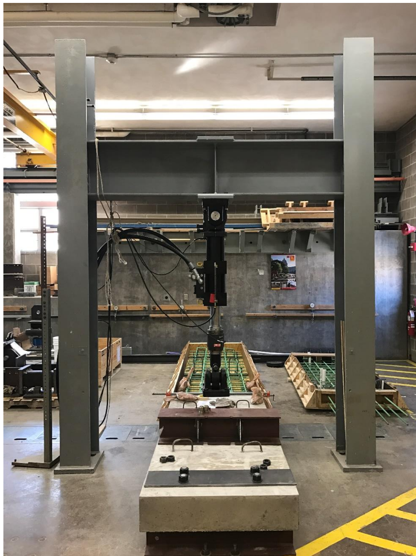
Figure 7.2 - Specimen in place underneath loading frame prior to casting of Stage 2 portion.
