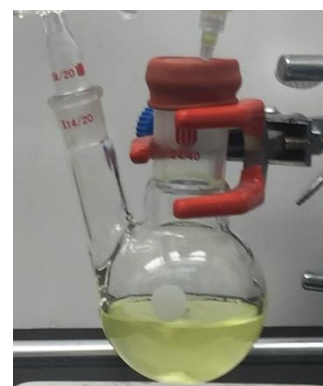
Figure 13: Trimethylsilyldiazomethane turns the methylating reaction yellow
