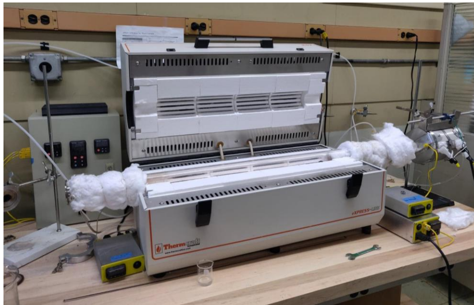
Figure 18. Complete steam furnace setup
