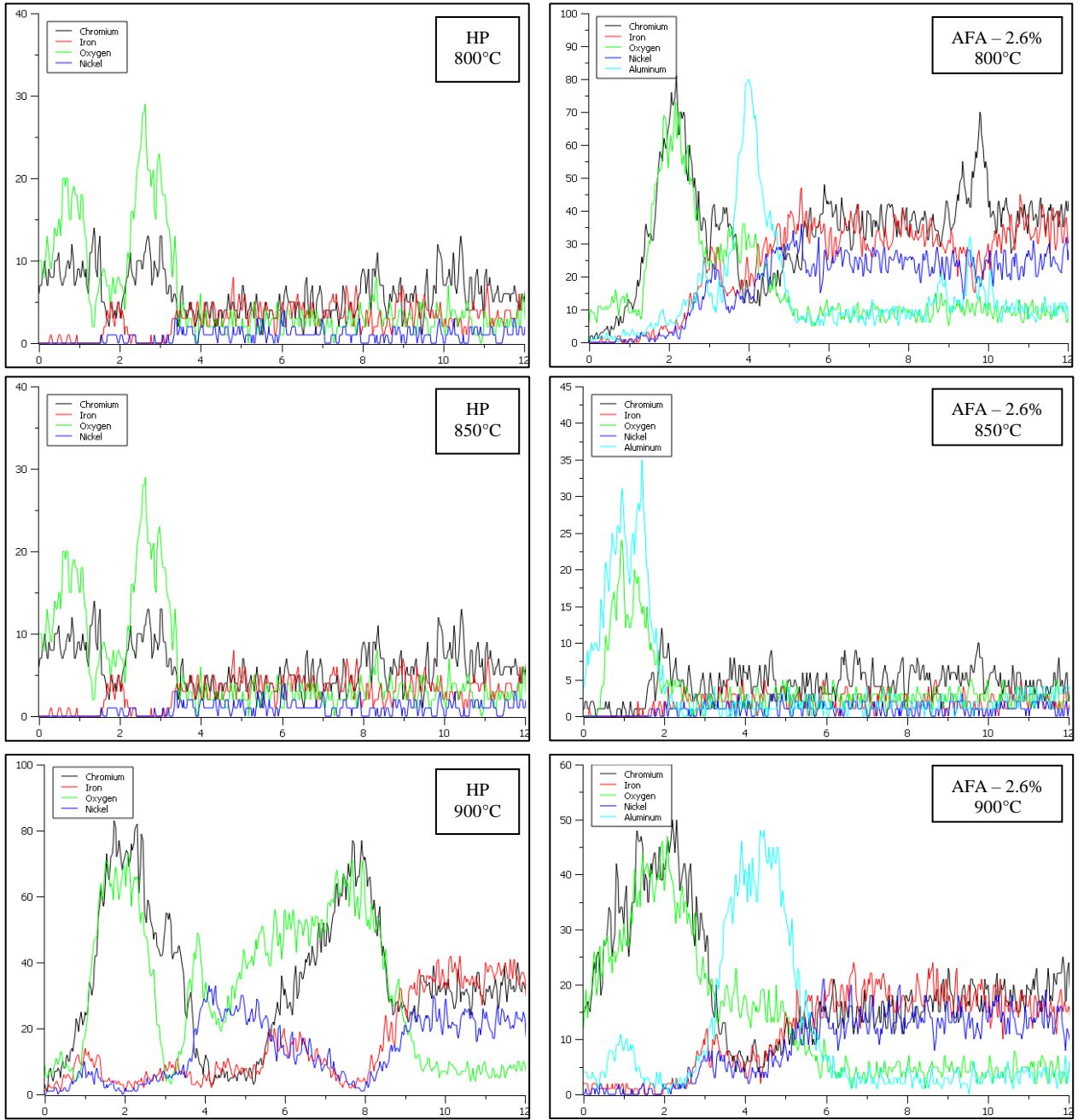
Figure 49. Line scans of AFA – 2.6% and HP at the 1:100 air-steam ratio.
