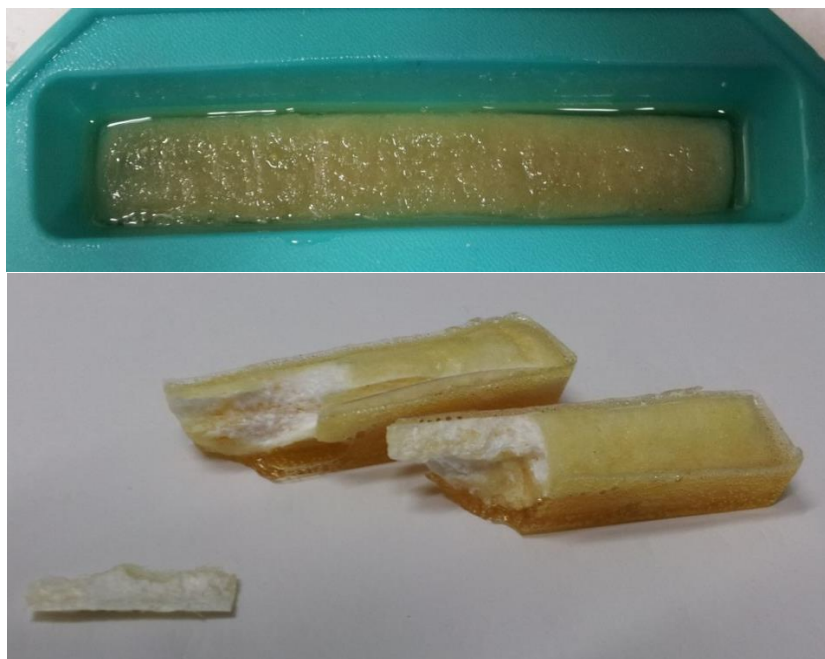
Figure 42 A photograph of an early trial of making a CNF/epoxy composite specimen using wet layup and a high viscosity resin. Incomplete wetting of CNF is seen in the lower image.
