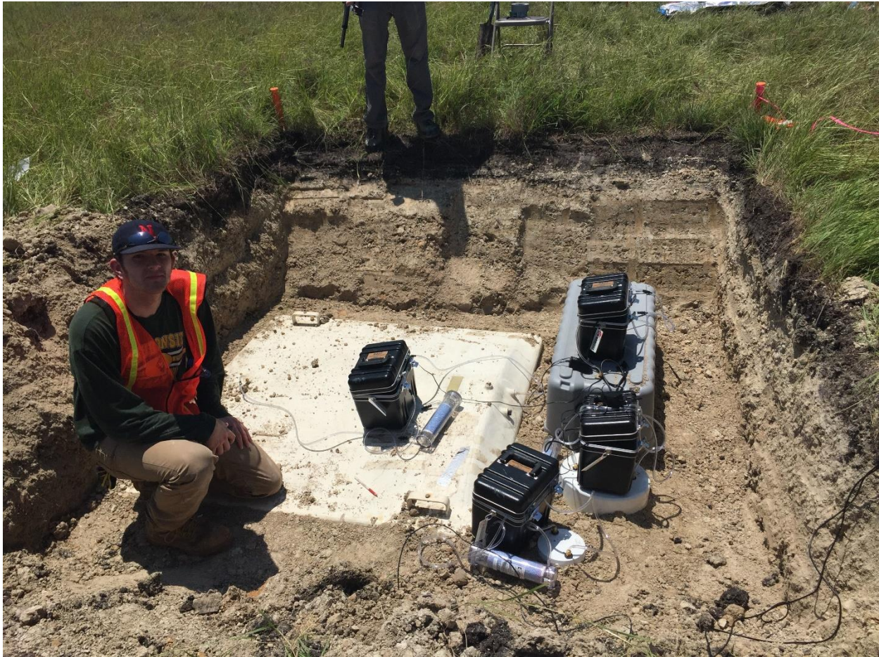
Figure A.6 General layout of each Test Pit with the large, medium, small, and extra small chambers measured Rn build up curves at the top of the Rn Barrier.
