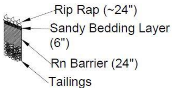
Figure A.1 Design Cross Section for the Falls City, TX UMTRCA cover system: (a.) top of cell, (b.) slope apron, and (c.) side slope.
