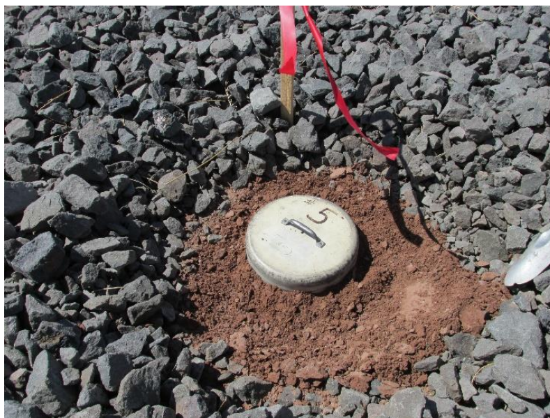
Figure 1.1 Photo of a 0.071 \text{ m}^2 Rn flux chamber passively accumulating radon with activated carbon. This is the standard practice currently used by UMTRCA guidelines.
