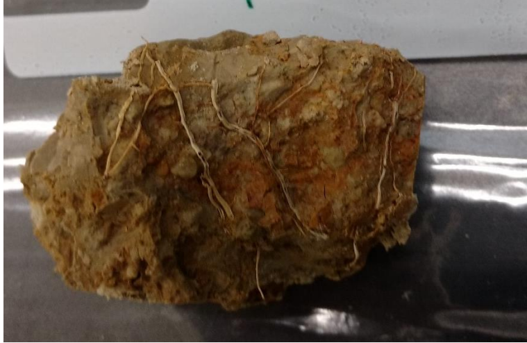
Figure A.18 Smaller roots, only 1 mm in thickness observed in the top of TP1A tube and throughout TP3A tube.
