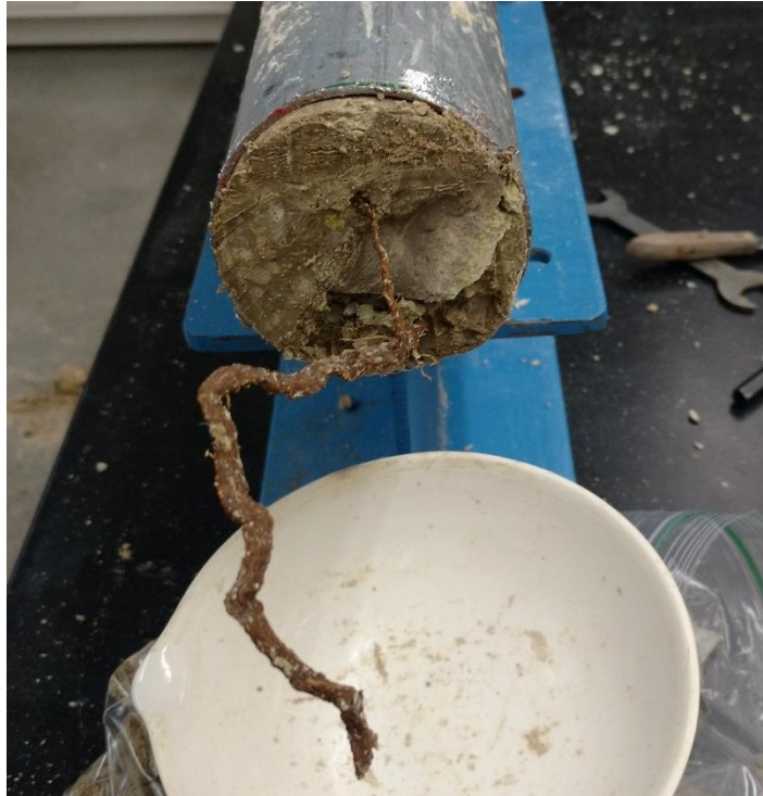
Figure A.19 Larger mesquite brush roots found in TP3A tube found 150 mm deep into the Rn barrier. Roots are about 5 mm in thickness.
