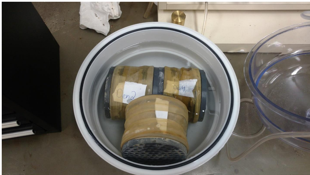
Figure 2.5 Three clay samples being prepared to be nearly fully submerged in a desiccator under vacuum to saturate for 24 h.
