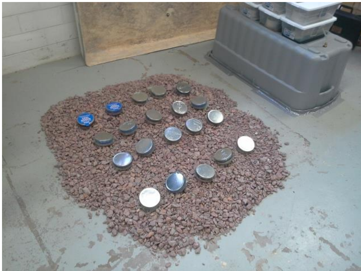
Figure 1.7 Experimental set up of AC canisters pre exposed to different RH ready to be exposed to Rn in the large chamber.
