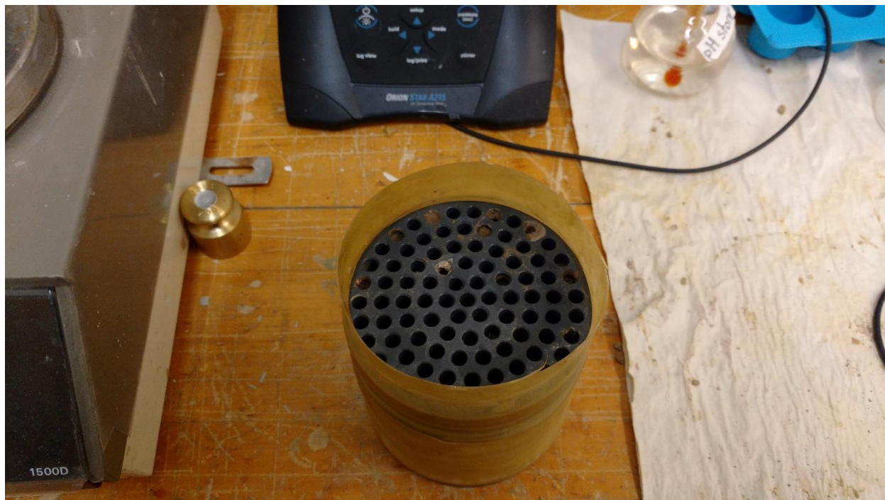
Figure 2.2 Testing apparatus used to provide a solid surface inside the permeamter.
