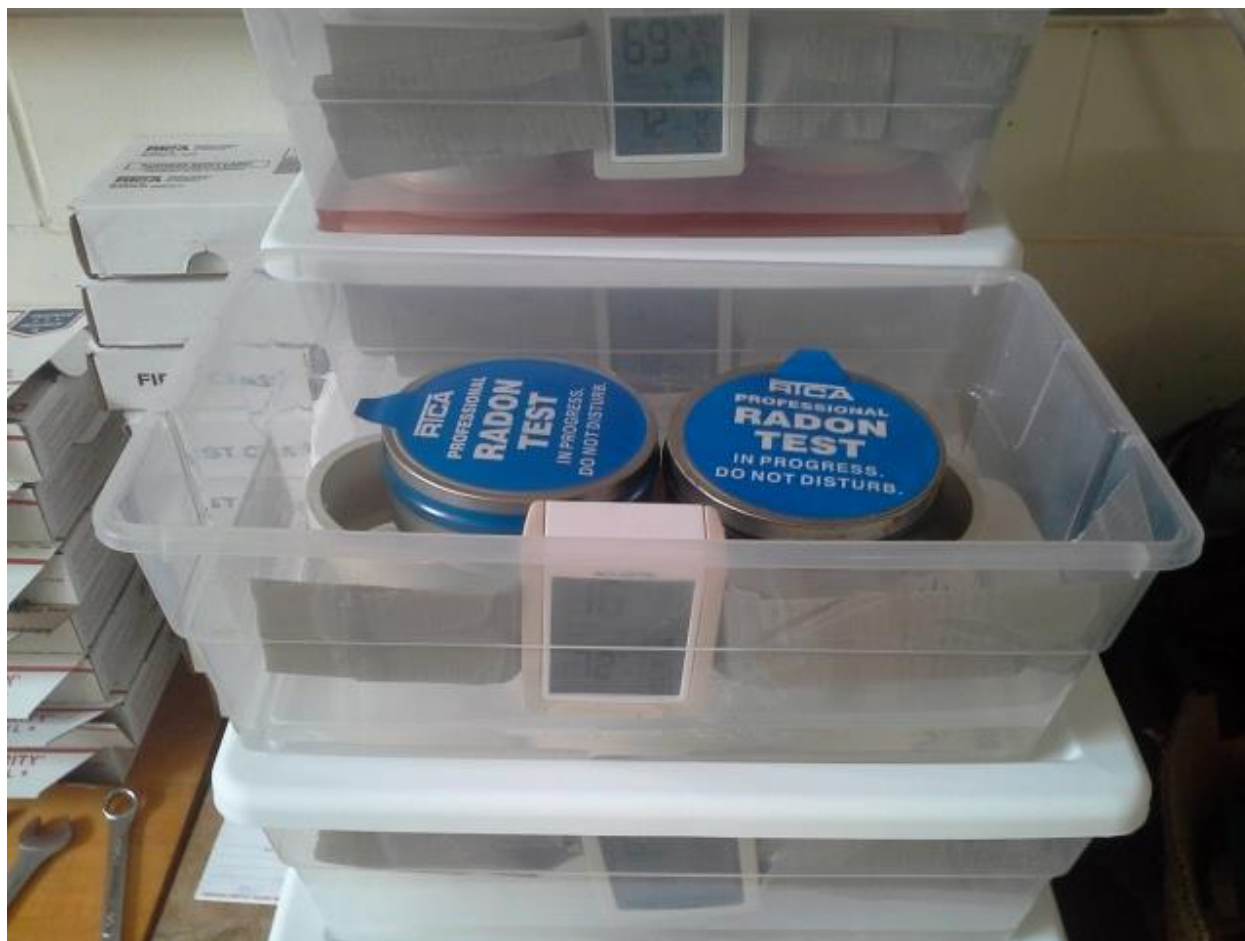
Figure 1.6 Two AC canisters placed in the chamber pre exposing them to RH. This chamber has RH of 16% due to the salt bath.
