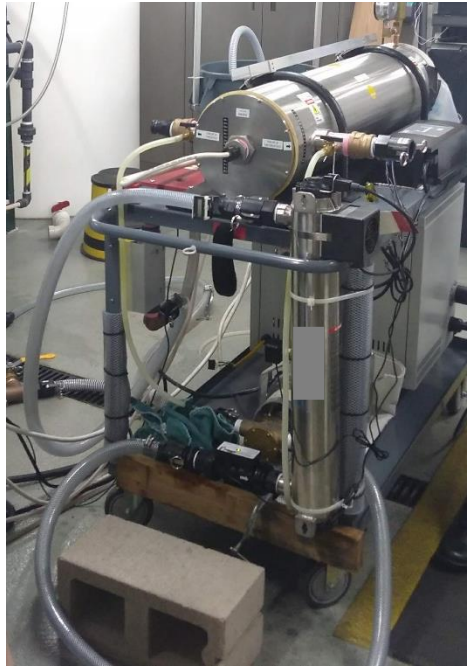
Figure 6. UV water purification system attached to the Amglo Kemlite BWMS cart.
