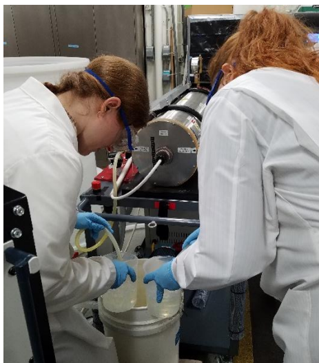
Figure 3. Collection of Algae and Microbe samples was made via control and treatment sample ports on the Amglo Kemlite treatment tank.
