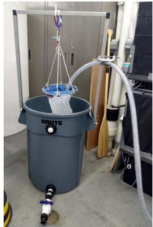
Figure 4. Effluent/Sampling tank with hose leading to collection net with solid 1 Liter cod end attached.
