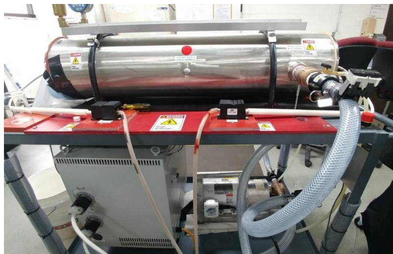
Figure 2. Amglo Kemlite Treatment tank, power supply and pump.
