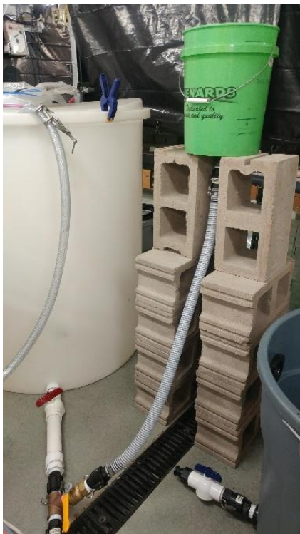
Figure 5. Zooplankton dosing bucket with hose leading to influent line of treatment tank.
