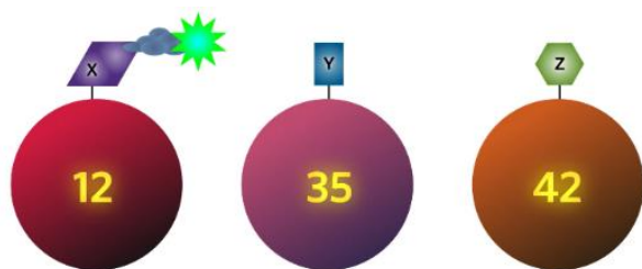
Figure 11: Structure of xMAP beads
