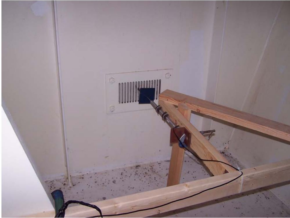
Figure 3.7: Longitudinal Expansion/Contraction LVDT
