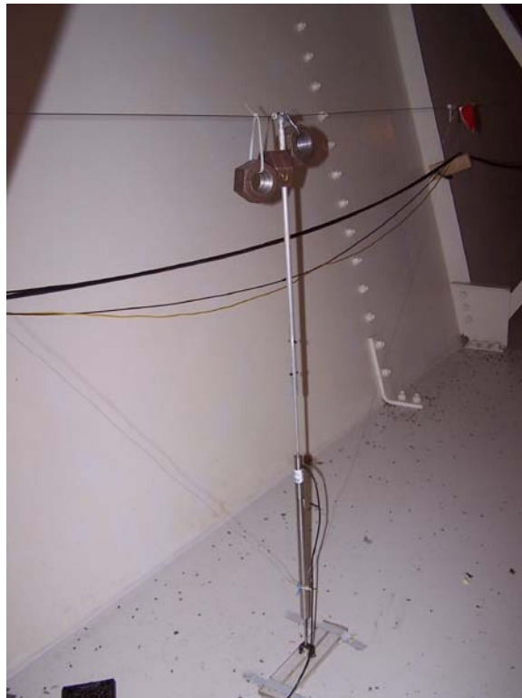
Figure 3.8: Mid-Span Deflection LVDT
