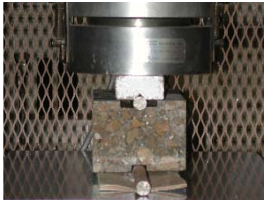
Figure 5.3.2 Photograph of the setup used for cracking specimens
