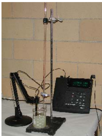
Figure 4.4.4 Beaker-electrode-buret assembly during a chloride ion analysis titration
