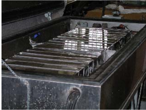
Figure 5.5.2 Freeze-thaw chamber at the WSMTL loaded with crack sealant specimens
