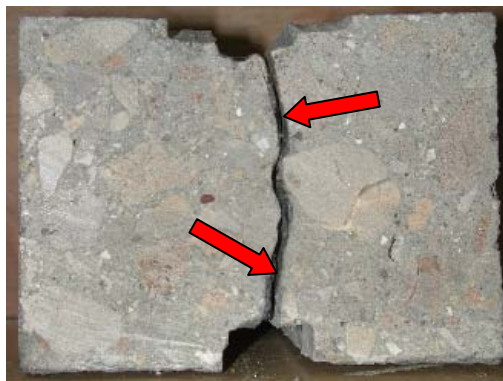
Figure 7.2.6 Example of a sealant failure during a bond strength test
