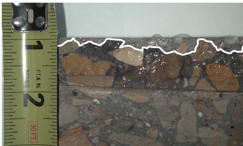
Figure 4.5.2 Depth of penetration profile measured on a trial specimen
