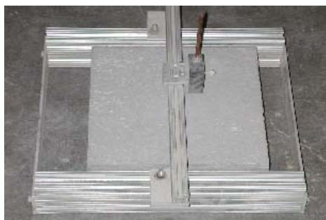
Figure 4.4.1 Sandblasting depth measurement device around specimen
