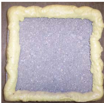
Figure 4.4.2 Sandblasted specimen with expansion foam dam ready to begin ponding
