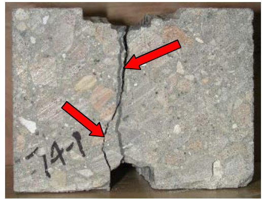
Figure 7.2.4 Example of a concrete failure during a bond strength test
