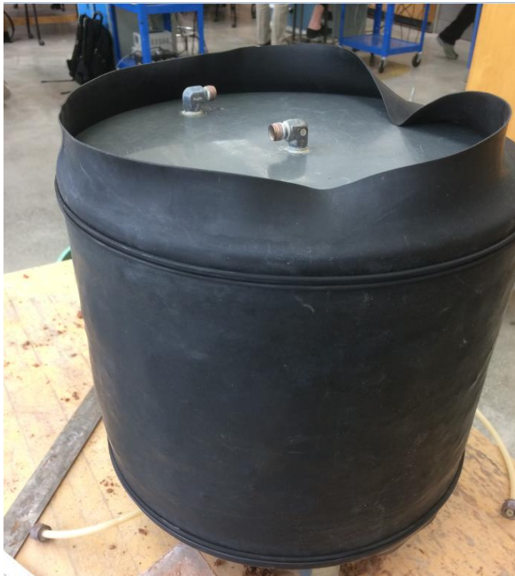
Figure 56 – 350 mm diameter block sample with flexible membrane installed for saturated hydraulic conductivity testing.
