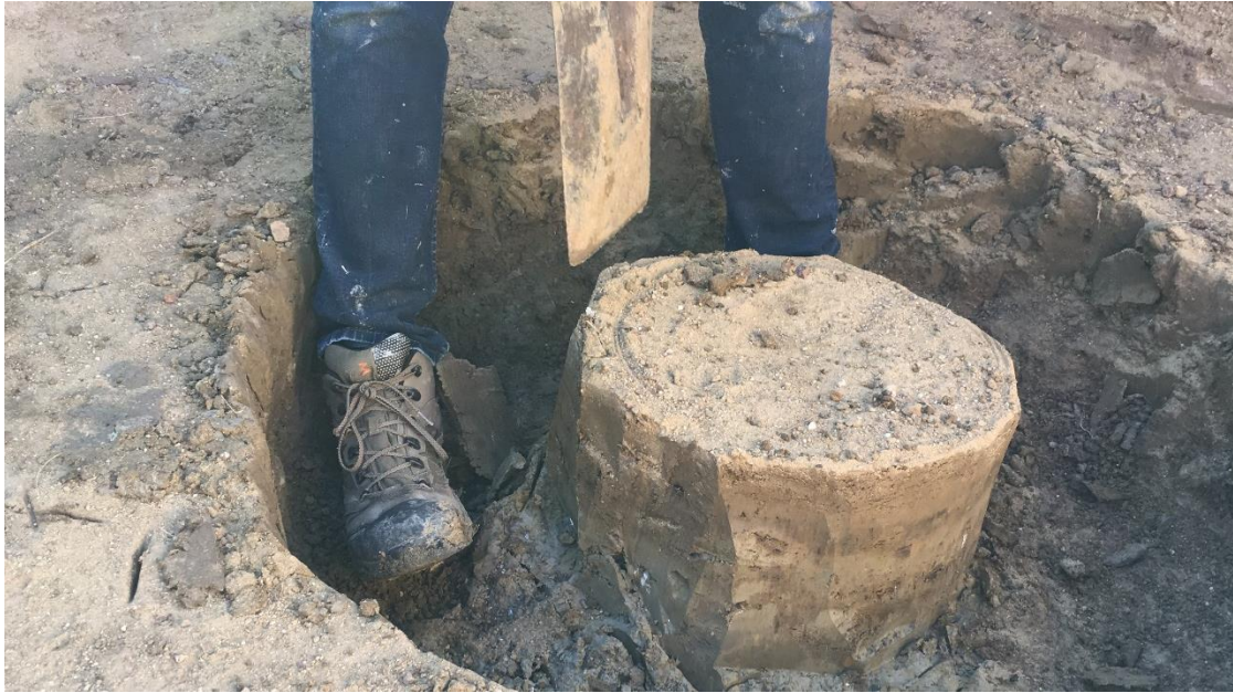
Figure D98 – Trimming a 350 mm diameter sample using a shovel.
