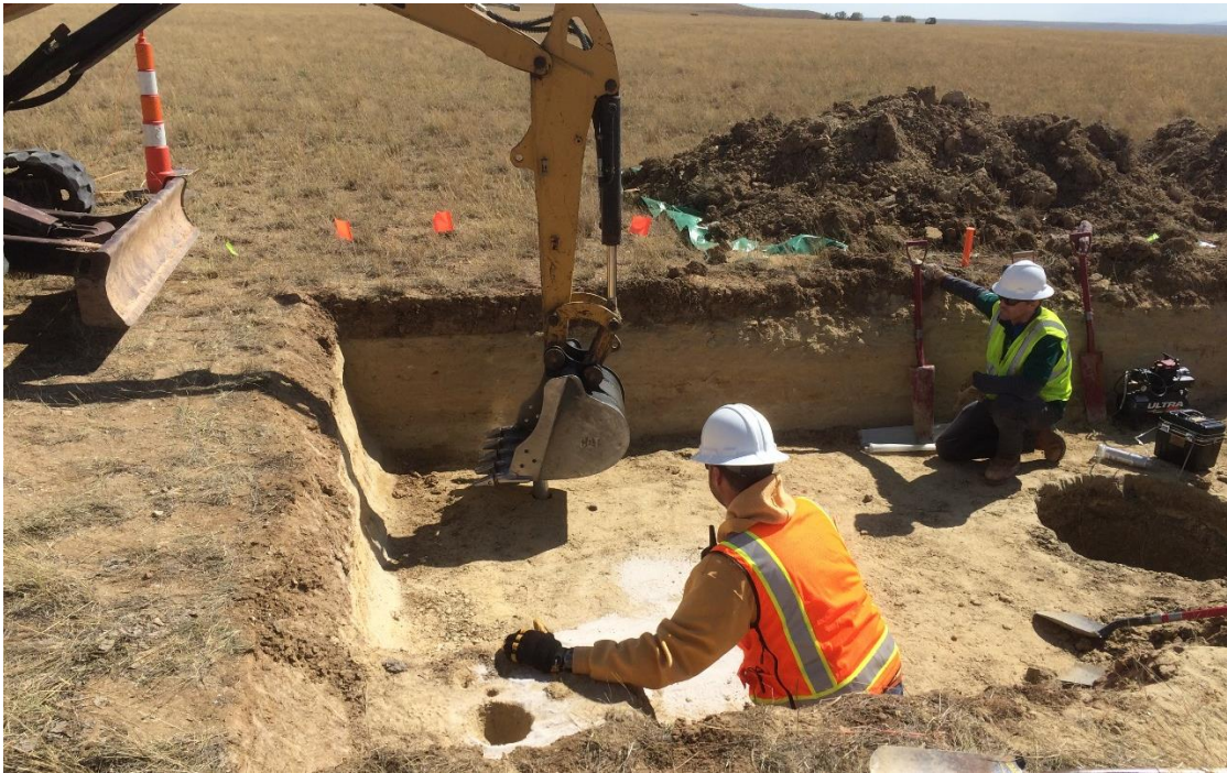
Figure D96 – Obtaining a thin-walled tube sample of Rn barrier soil.
