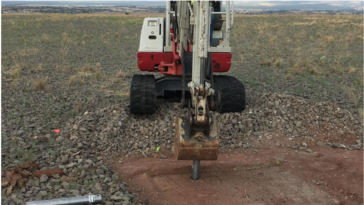
Figure 50 – Obtaining a thin-walled tube sample of Rn barrier soil.
