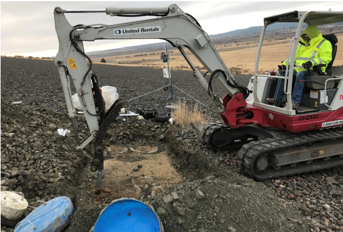
Figure 139 - Obtaining a thin-walled tube sample of Rn barrier soil.
