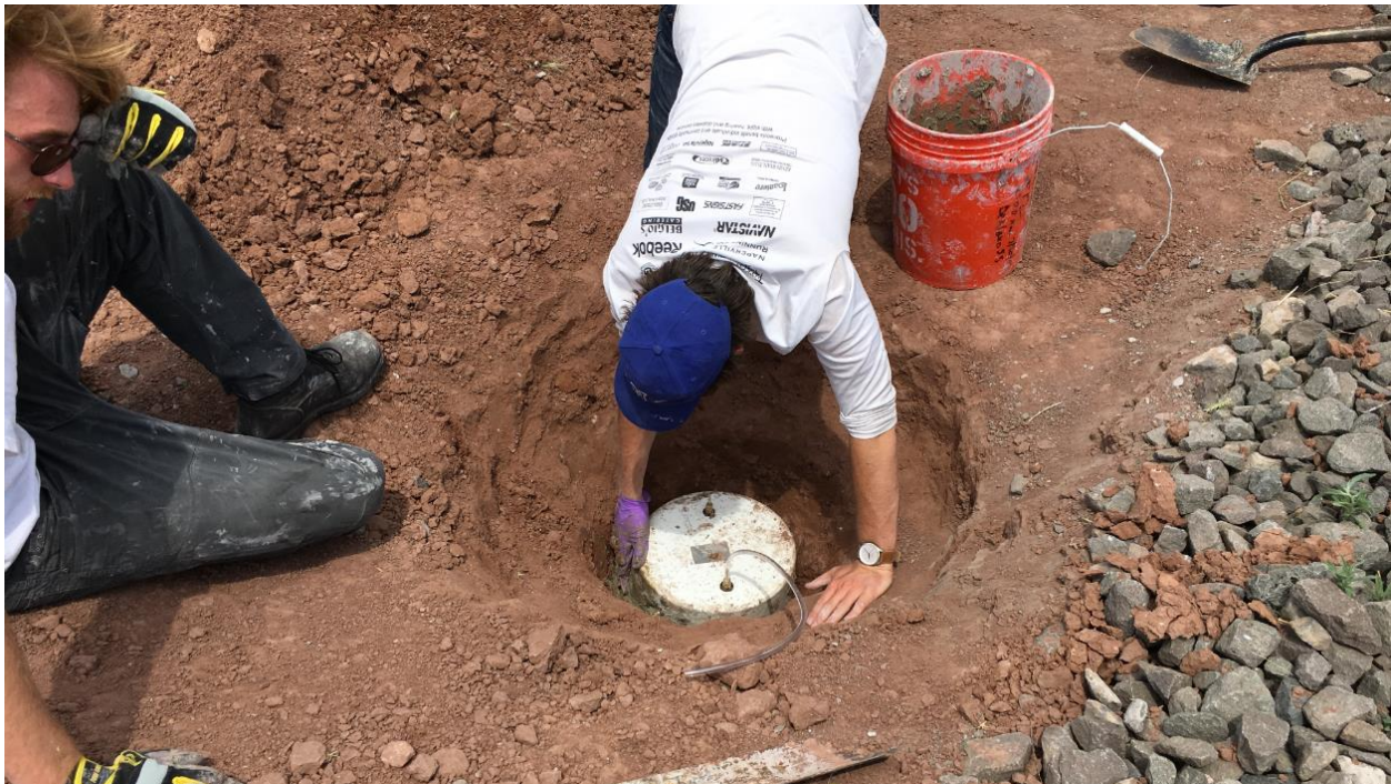
Figure 49 – Installation of a small flux chamber on the exposed tailings.
