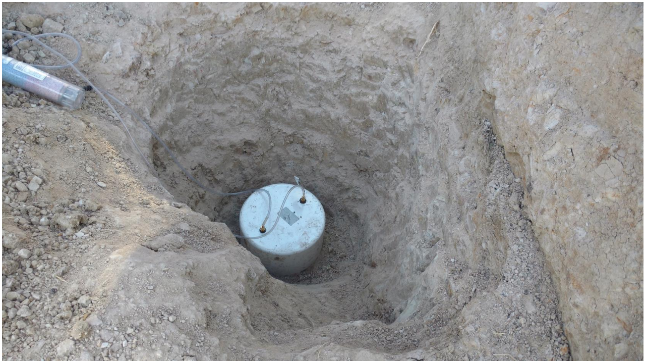
Figure 14 – Small flux chamber placed directly on tailings.
