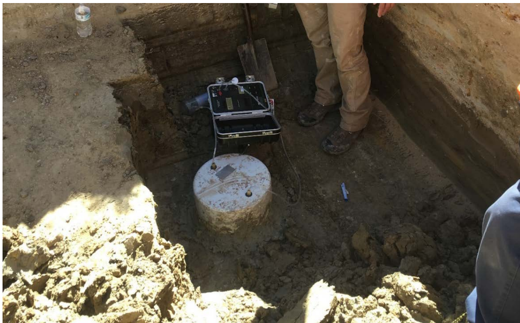
Figure 4.10 – A small flux chamber installed directly on the tailings.
