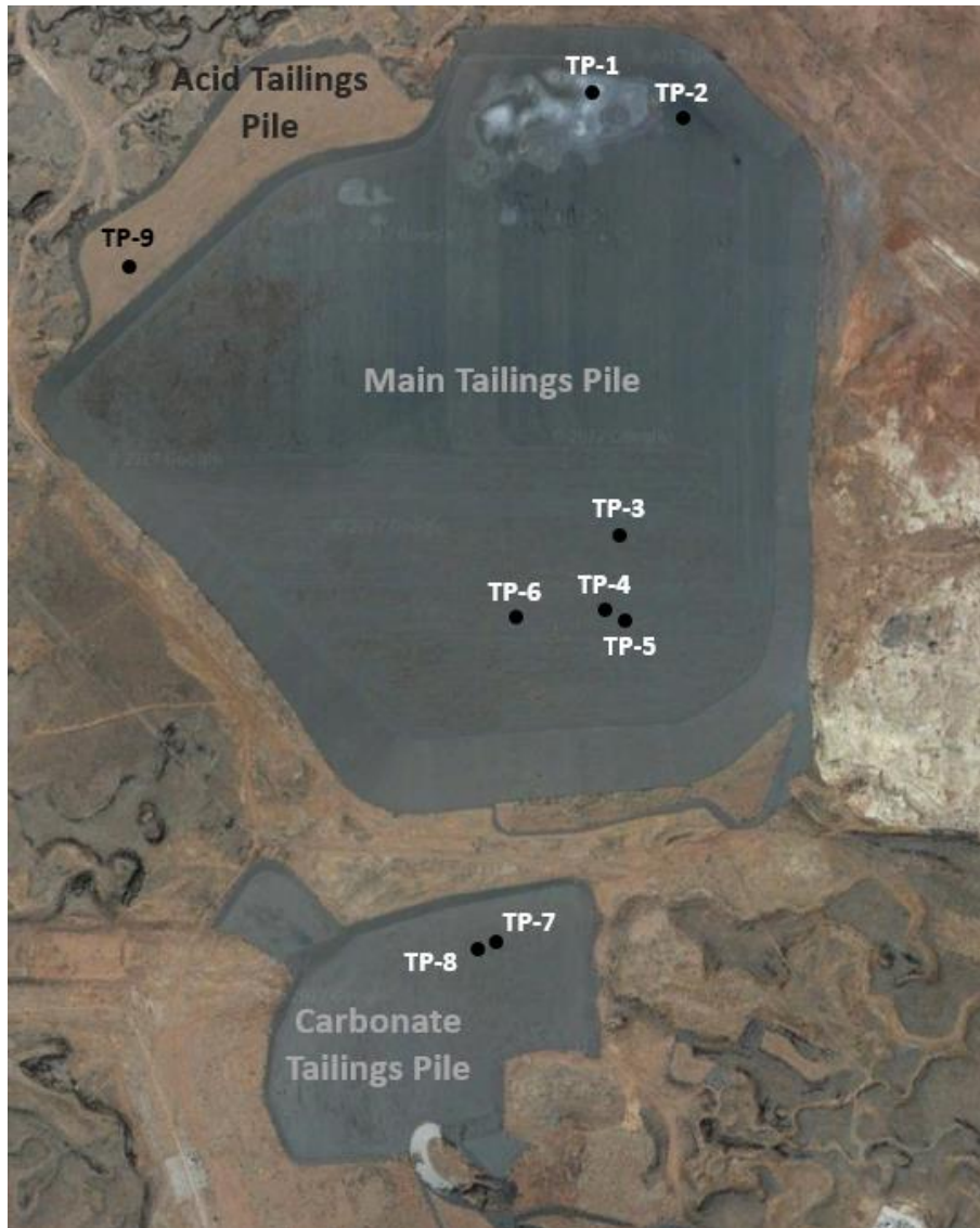
Figure 45 – Approximate locations of test pits excavated at the Bluewater, NM site.
