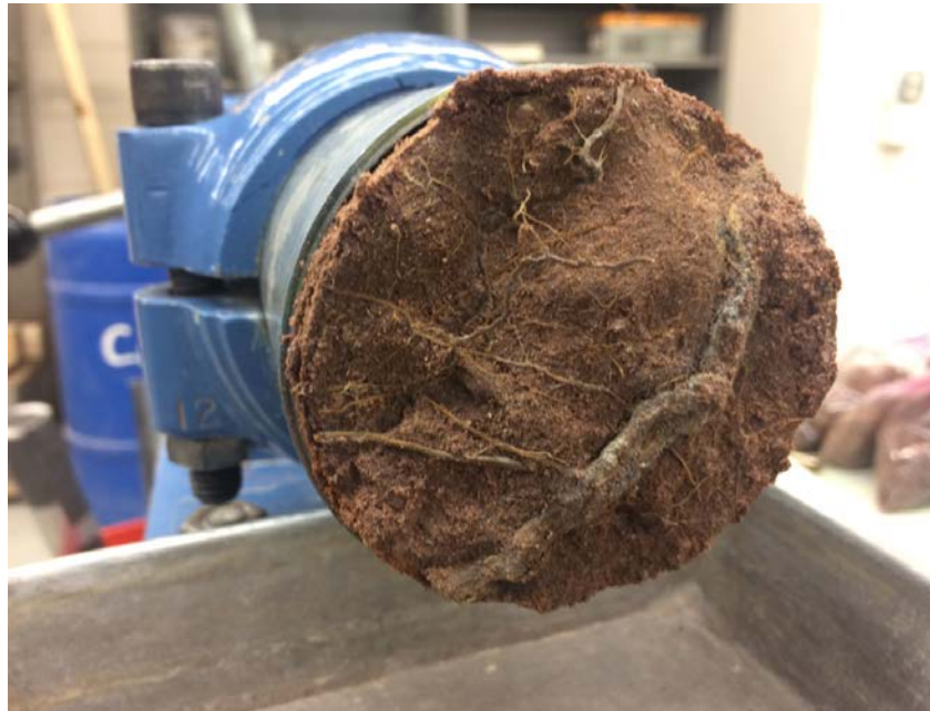
Figure 5.1.13 – Large root in 70 mm diameter Shelby tube sample from Bluewater, NM test pit 5.
