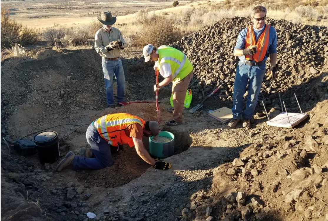
Figure 140 – Trimming a 350 mm diameter block sample using a shovel.
