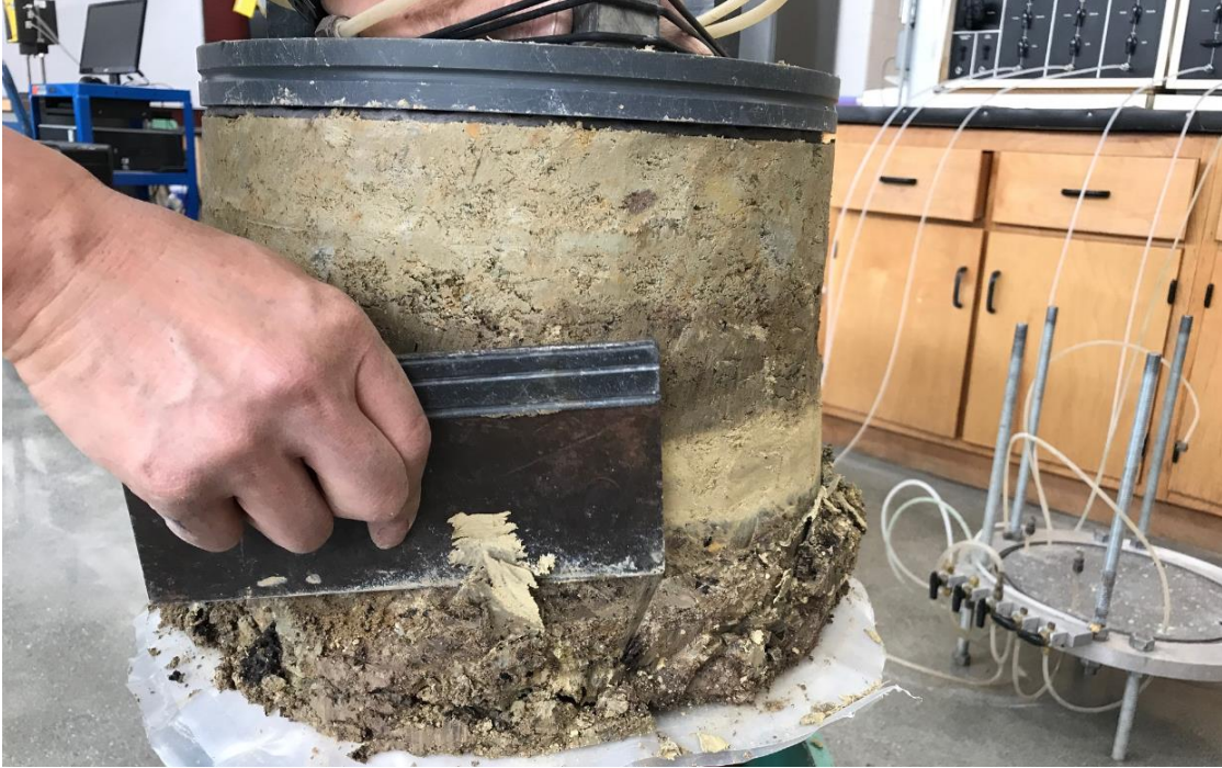
Figure D102 – Trimming a 350 mm diameter block sample prior to saturated hydraulic conductivity testing in the laboratory.
