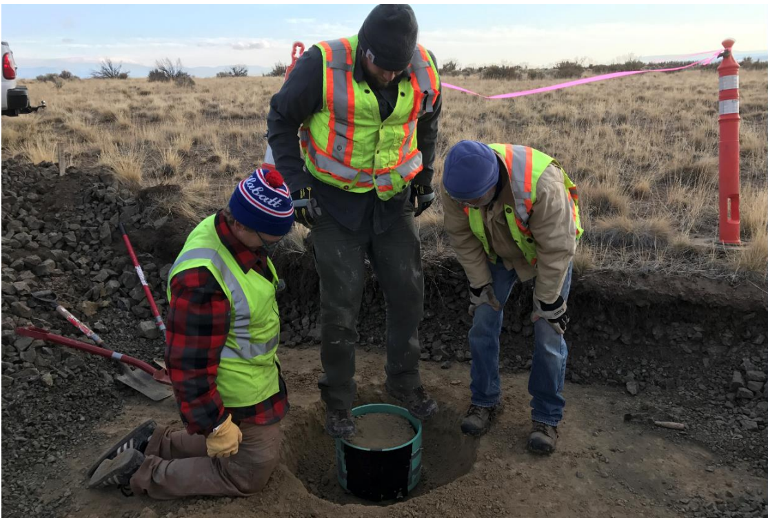
Figure 141 – Installing a protective PVC sleeve around a 350 mm diameter sample.
