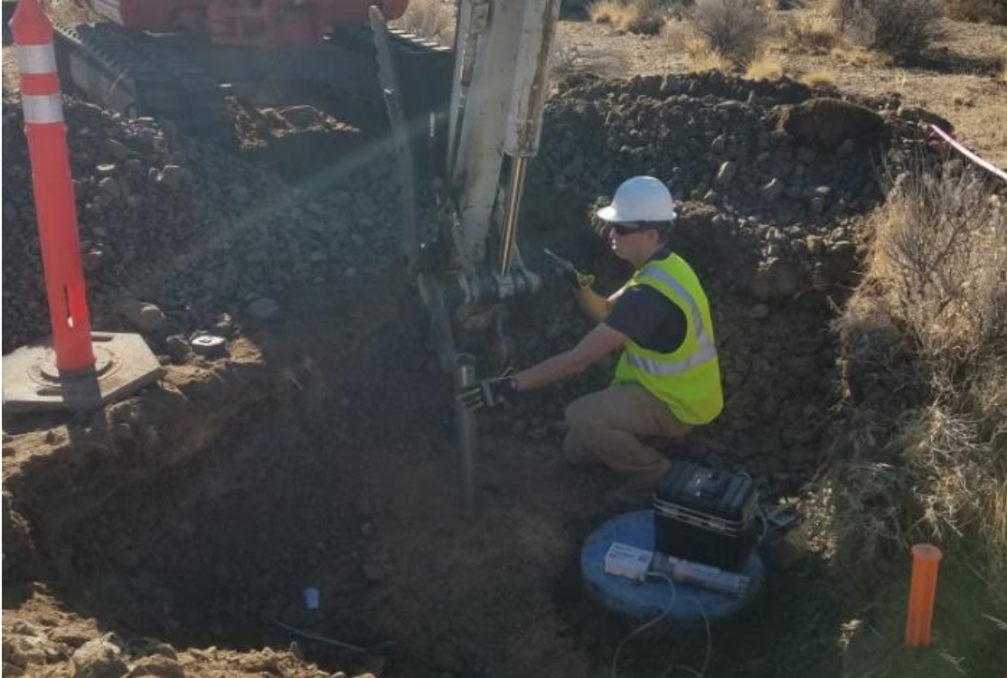
Figure 138 – Obtaining a thin-walled tube sample of Rn barrier soil.
