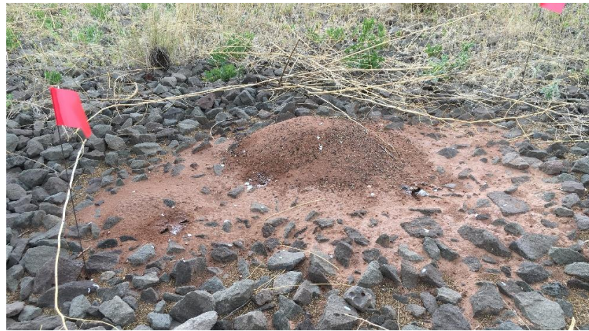
Figure 37 – Clockwise from top left: 1. Unvegetated riprap erosion cover. 2. Grasses growing in the riprap cover layer. 3. Ant mound protruding from the riprap cover (Test Pit 6). 4. Salt bush growing from the riprap layer (ATV for scale).
