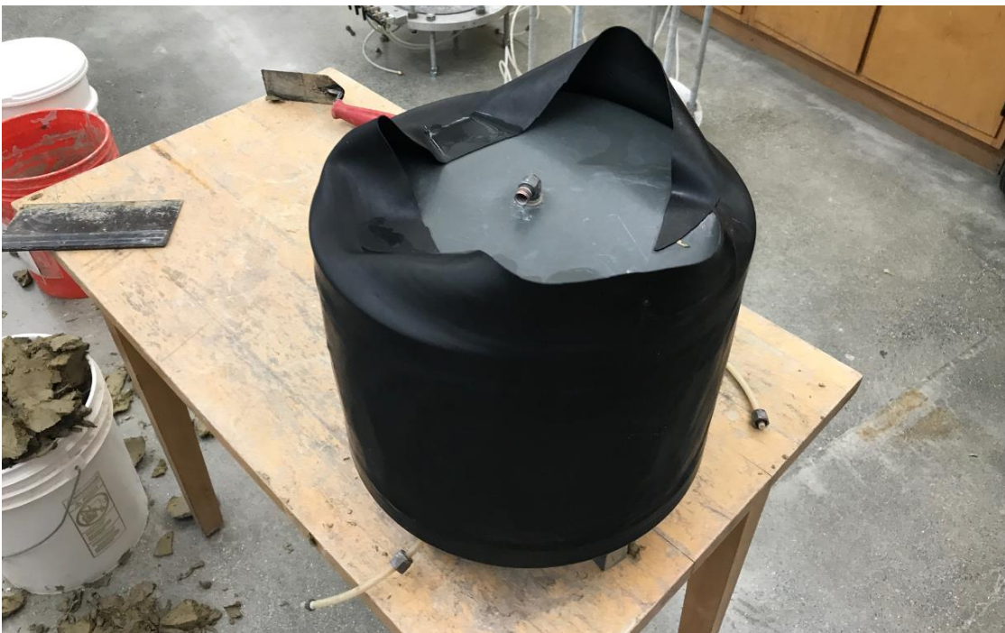
Figure D103 - A 350 mm diameter block sample with flexible membrane in place prior to saturated hydraulic conductivity testing in the laboratory.
