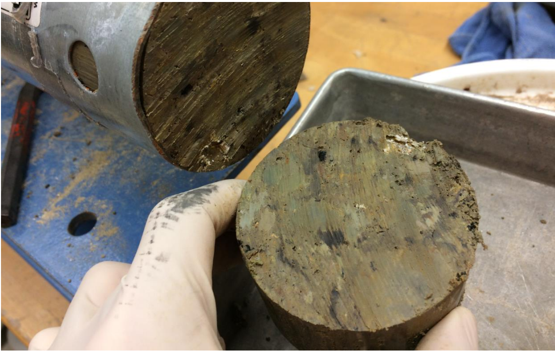
Figure D97 – Sampling soil from a thin-walled tube in the laboratory.
