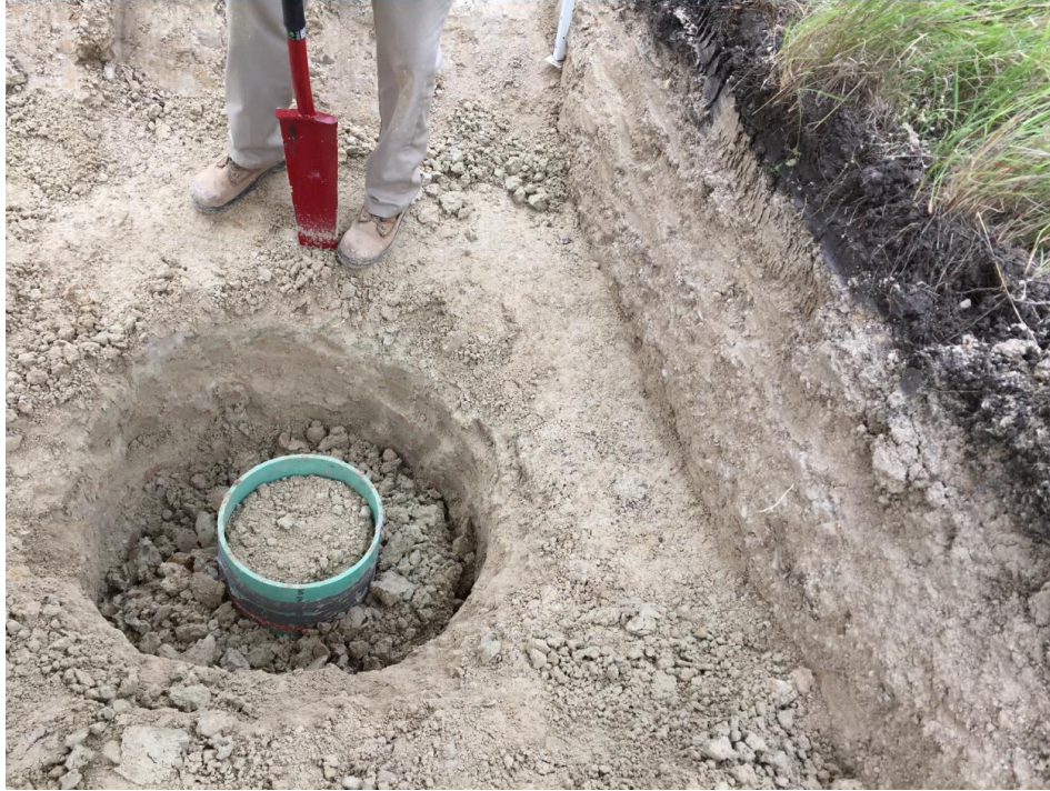
Figure 16 – Excavating a 350 mm diameter block sample using a shovel.
