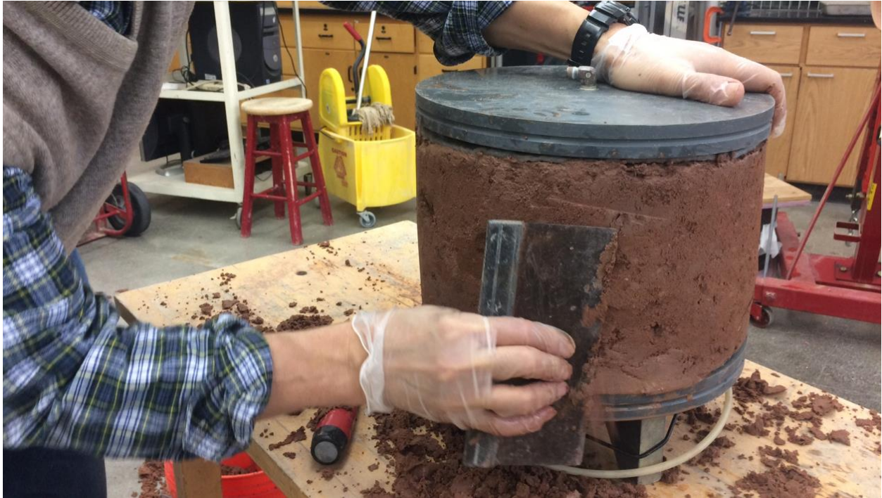
Figure 55 – Trimming 350 mm diameter block sample for saturated hydraulic conductivity test.
