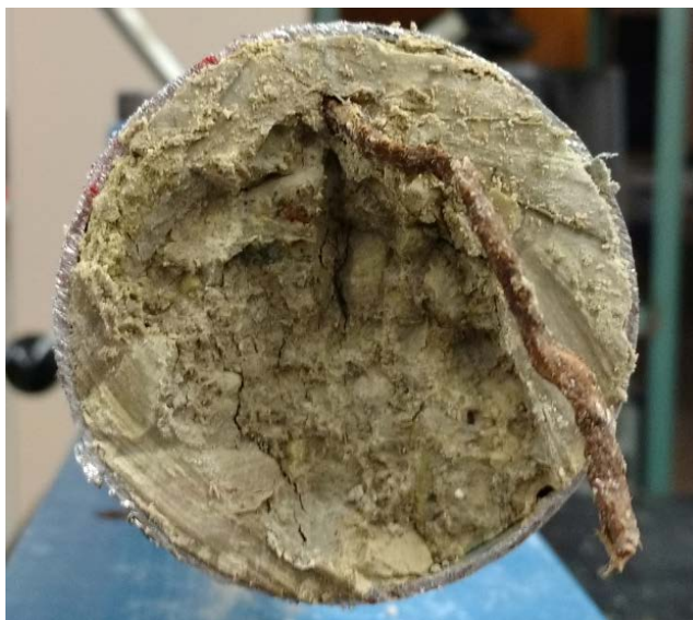
Figure 5.1.11 – A large root protruding from a thin-walled Shelby tube sample from TP-3 from Falls City, TX.
