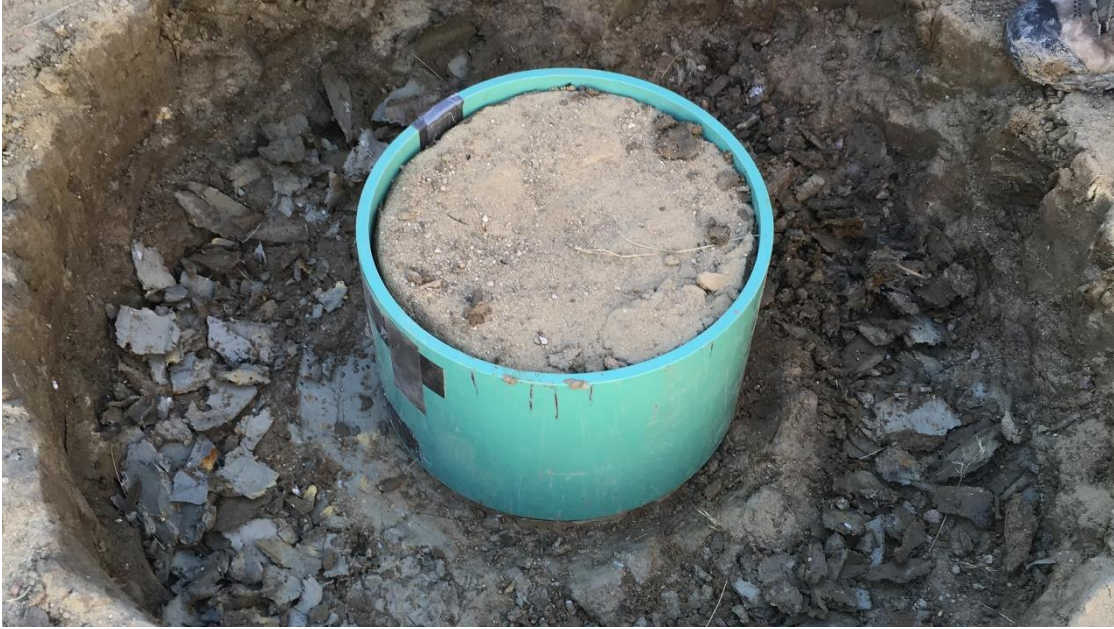
Figure D100 – 350 mm diameter sample with protective PVC pipe in place.
