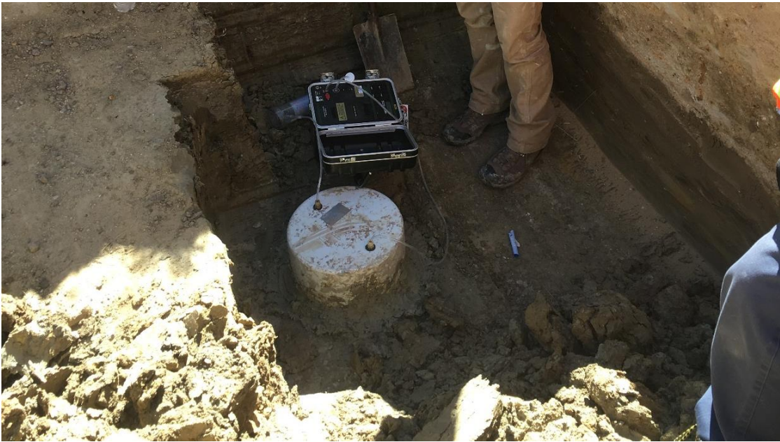
Figure C95 – Installation of a small flux chamber directly on the uranium mill tailings.
