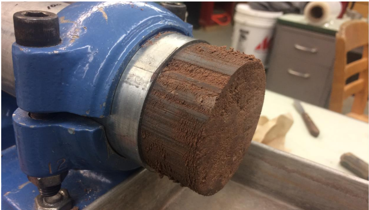
Figure 51 – Extraction of a 70 mm diameter (Shelby) tube sample in the lab.
