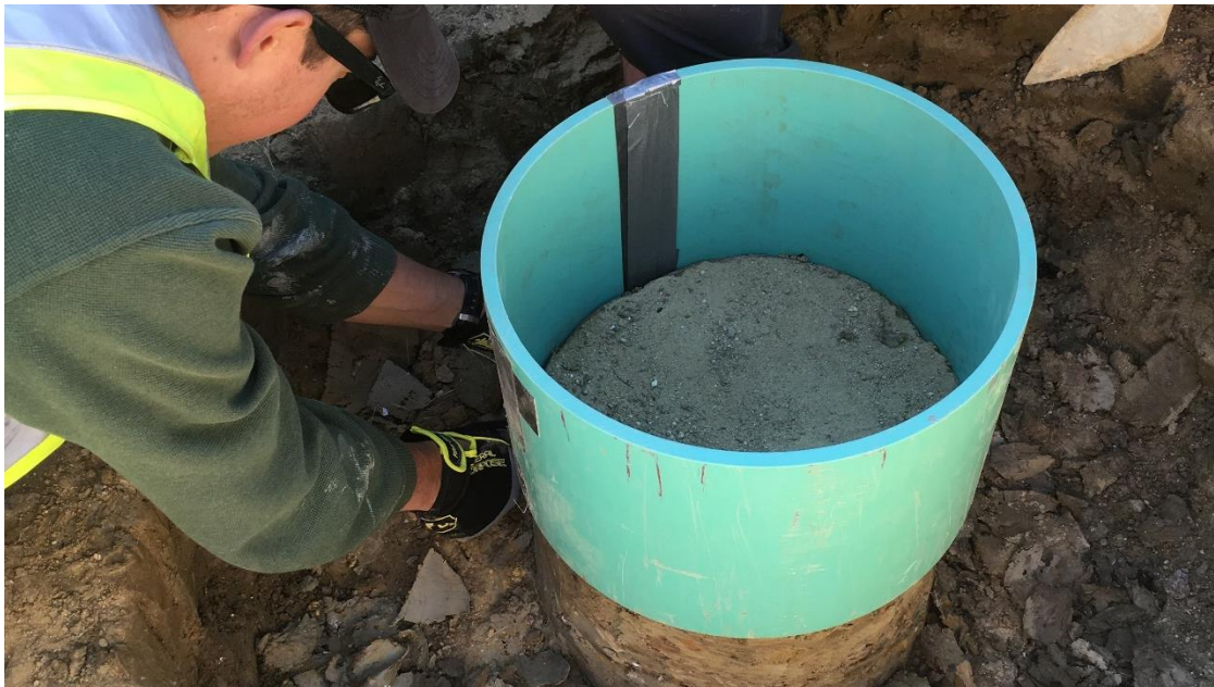
Figure D99 – Trimming a 350 mm diameter sample using hand tools to fit protective PVC pipe around sample.
