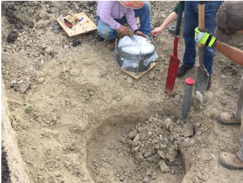
Figure 17 – Securing the excavated 350 mm diameter block sample in a protective casing.
