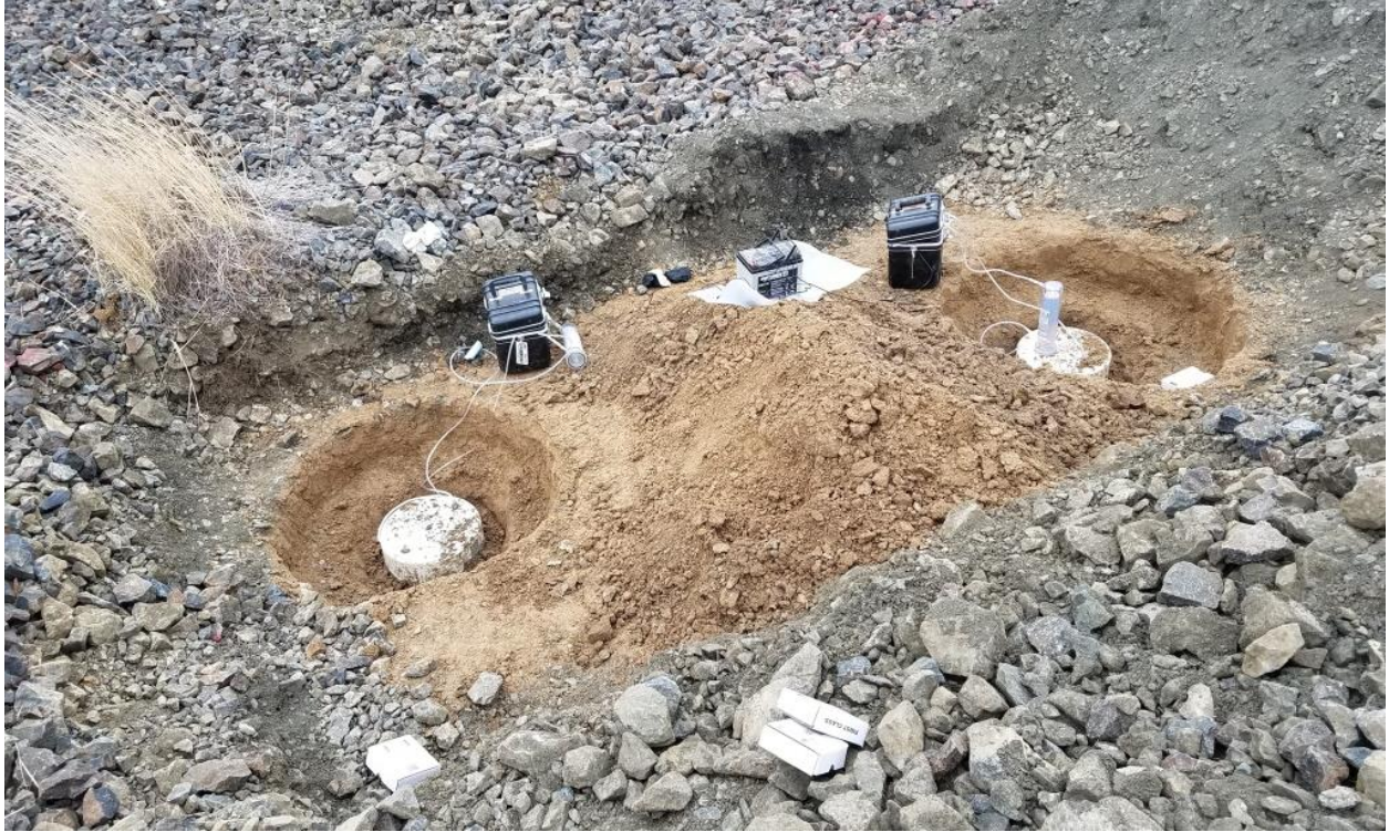
Figure 137 – Flux chambers installed on exposed tailings.
