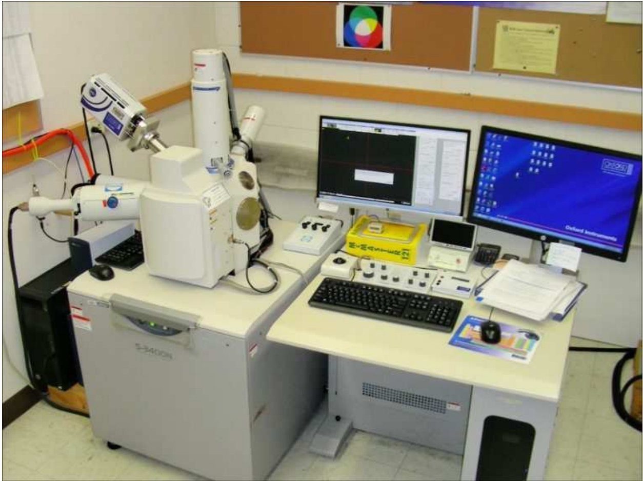
Figure 9: The Hitachi S3400 Variable Pressure Scanning Electron Microscope with the Oxford EBSD detector (on the left). The computer software is used to select the location in the thin section that will be indexed.
