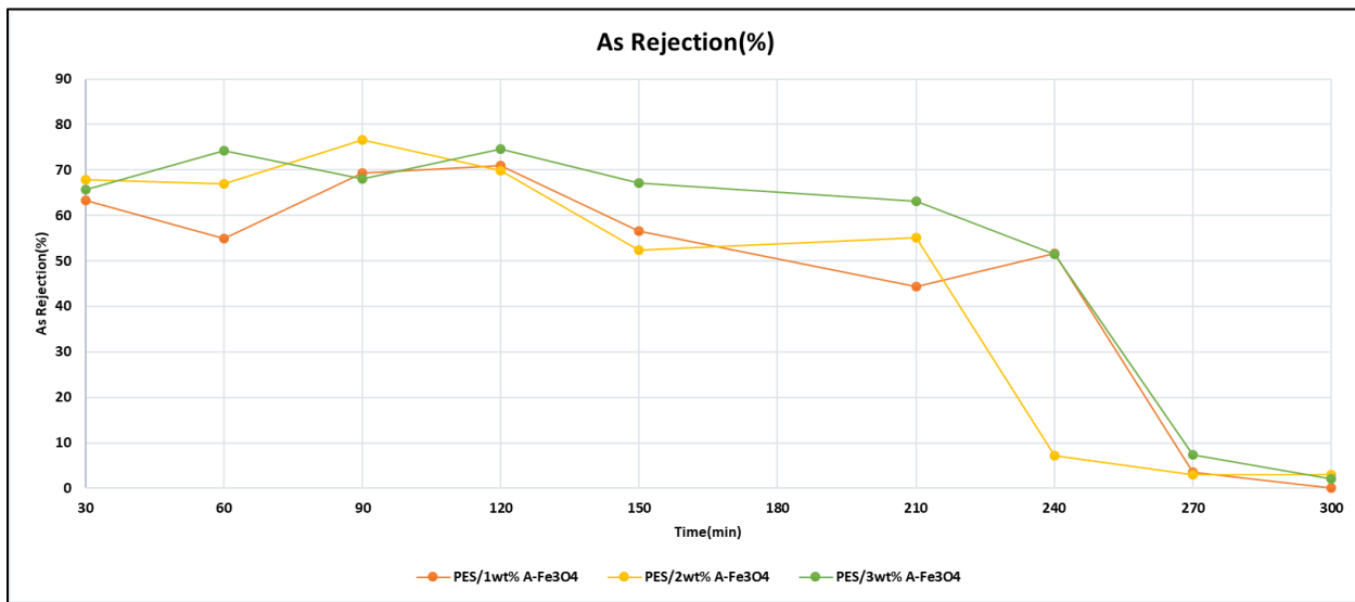
Figure 3.17 Prepared Membranes (M2, M3, M4) As(V) ion rejection at 50psi
