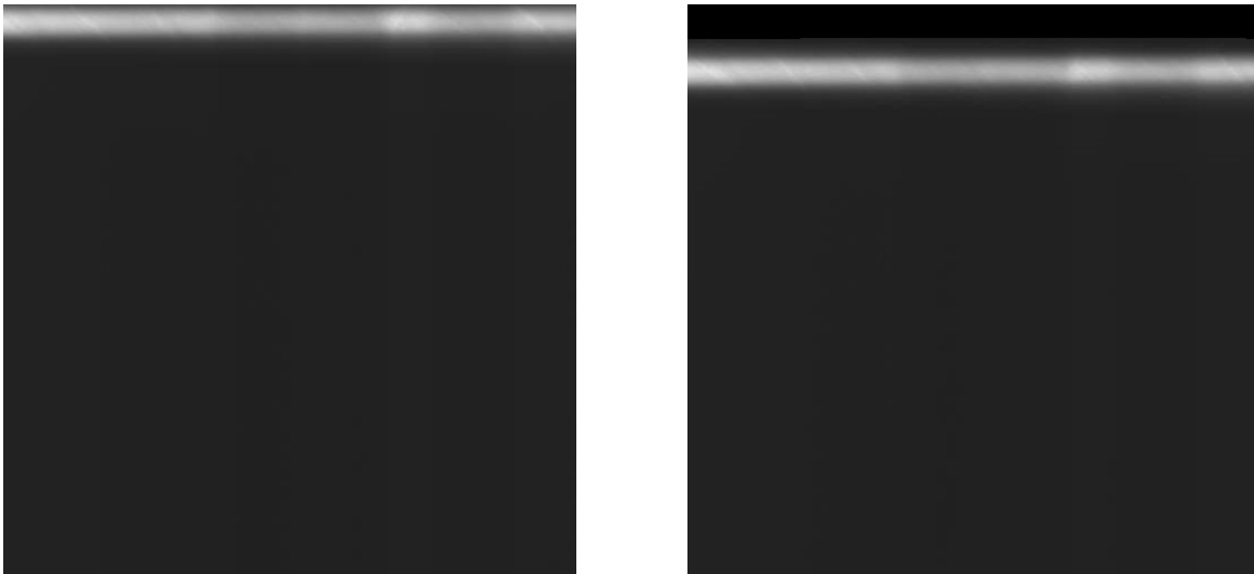
Figure 4-7. Fast kinetics acquisition process. An image is taken at the very top of the CCD, and its charge is then shifted down. This leaves the original sub area clear to acquire a new image.
