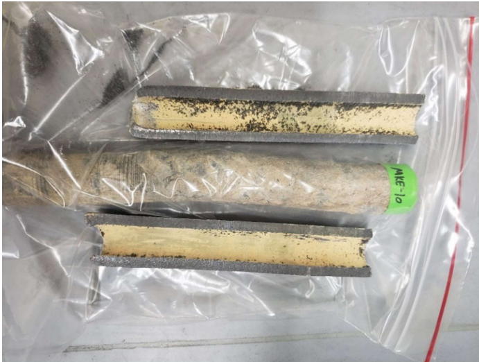
Figure A-22. Longitudinal cross-section of MKE-10 lead lateral pipe displaying tan colored corrosion scales on the inner pipe wall, which are common within lead carbonate minerals.
