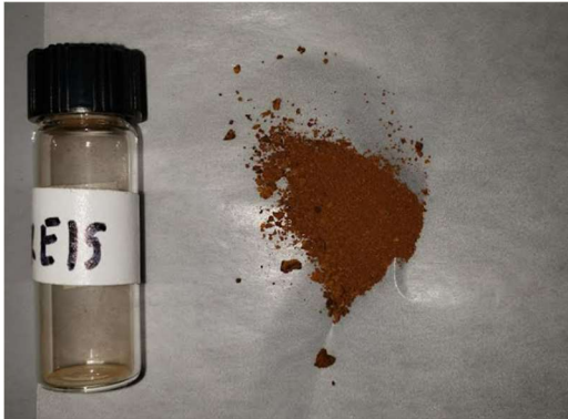
Figure A-33. Powderized corrosion scale scraped from the inside of a cast iron main in Milwaukee.
