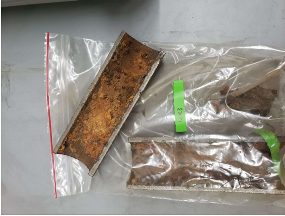
Figure A-57. Cross-section of an iron pipe section obtained from Waukesha.
