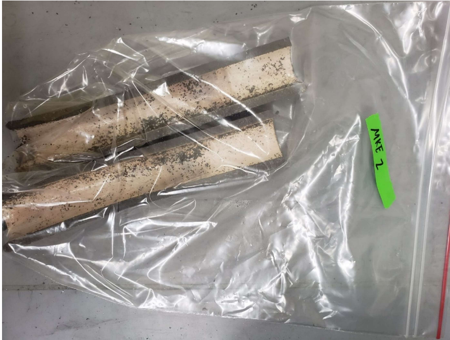
Figure A-3. Longitudinal cross section of MKE-2 lead pipe.
