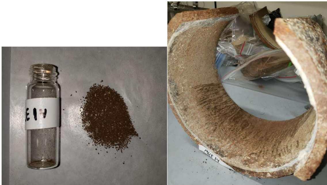
Figure A-31. Powderized corrosion scale scraped from the inside of a ductile iron drinking water lateral harvested from Milwaukee.
