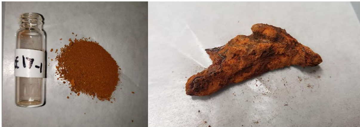
Figure A-37. Powder scraped from the inside pipe wall of a cast iron main in Milwaukee. A chunk deposit is shown on the right.
