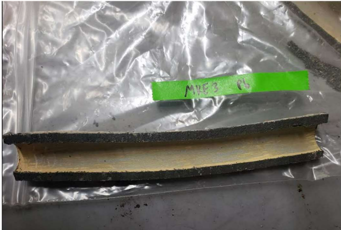
Figure A-6. Longitudinal cross section of MKE-3 lead pipe. Inner walls of the pipe were a tan color, characteristic of lead carbonate minerals.
