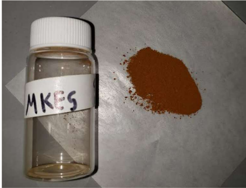
Figure A-10. MKE-5 powder sample scraped from a cast iron drinking water pipe in Milwaukee.
