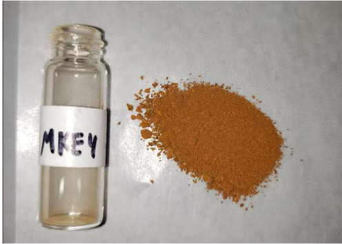
Figure A-8. MKE-4 powder sample scraped from a cast iron corrosion scale on a Milwaukee drinking water pipe.
