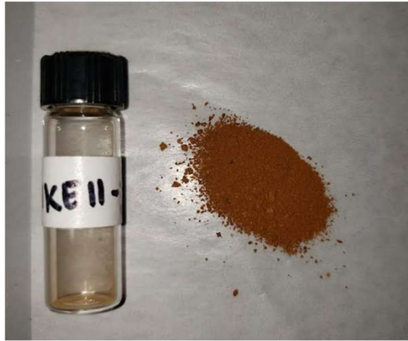
Figure A-24. Corrosion scale powder from a cast iron drinking water main in Milwaukee.
