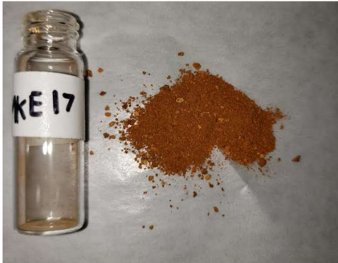
Figure A-35. Powder obtained from scraping the corrosion scale from a cast iron main in Milwaukee.
