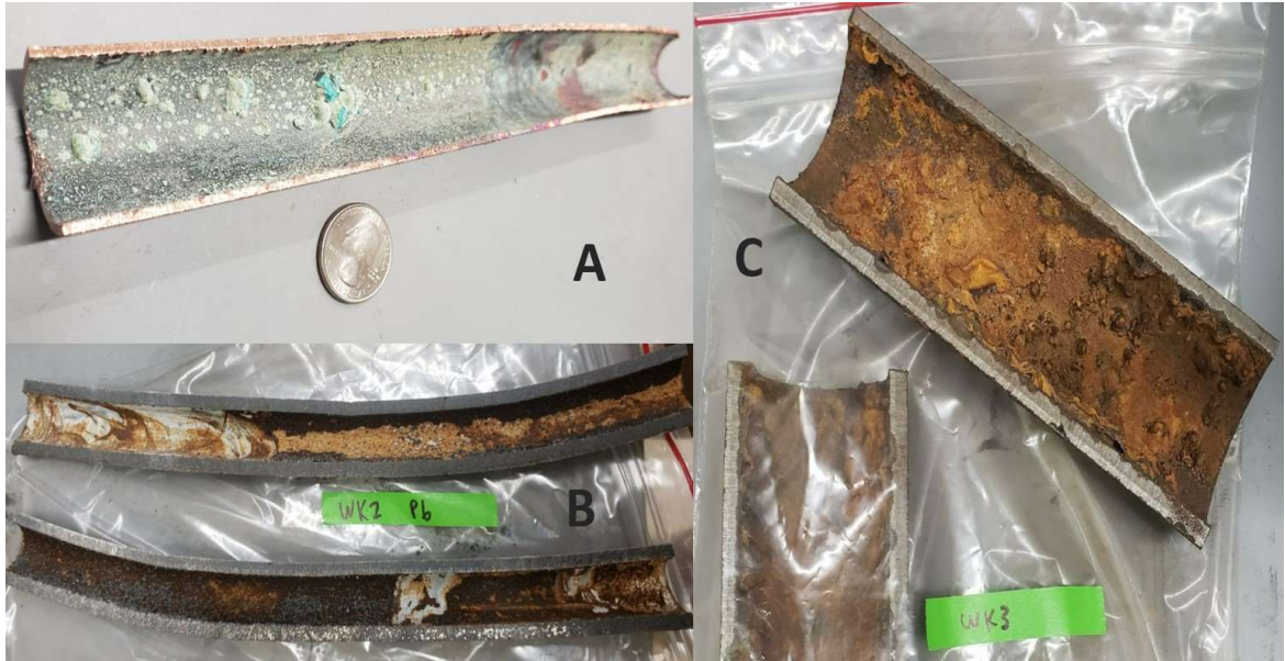
Figure 4-5. Longitudinal cross sections displaying corrosion scales from copper (A), lead (B), and iron (C) pipes.
