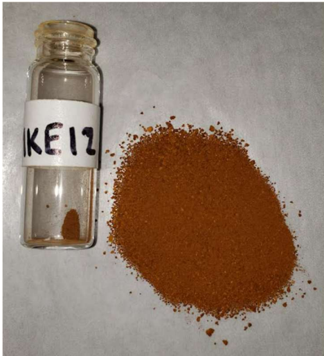
Figure A-26. Corrosion scale powder scraped from the inside pipe wall of a cast iron drinking water main in Milwaukee.
