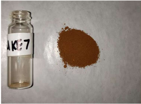
Figure A-15. MKE-7 powder sample scraping from a scale in a cast iron drinking water pipe from Milwaukee.
