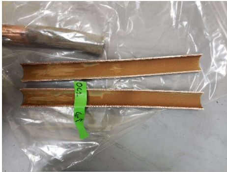
Figure A-40. Cross section of a copper lateral obtained from Oak Creek.
