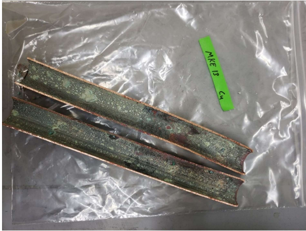
Figure A-28. Longitudinal cross section of a copper lateral harvested from Milwaukee. Corrosion accumulation is shown as green-blue buildup on the inside of the pipe walls.
