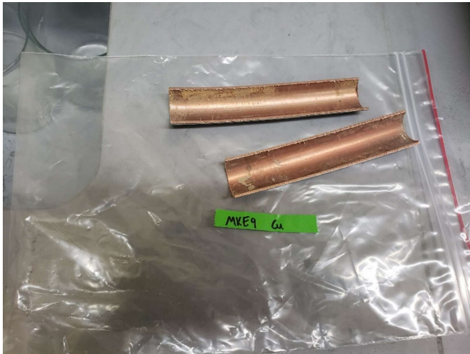
Figure A-17. Longitudinal cross-section of a copper drinking water pipe from Milwaukee displaying minimal corrosion scaling.
