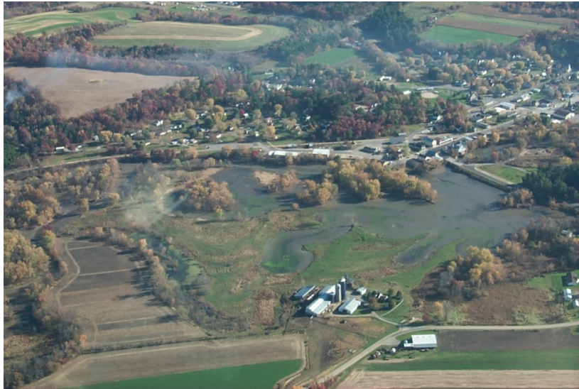
Figure 37 Photo courtesy of Emily Stanley and Martin Doyle. Picture of La Valle dam reservoir during the January 1999 drawdown, approximately one year before removal. River flows from left side of picture towards the right side of picture.
