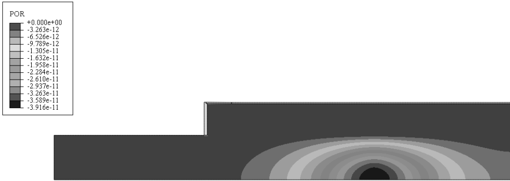
Figure 5.91 Distribution of excess pore pressure at the end of the analysis ( psf )
