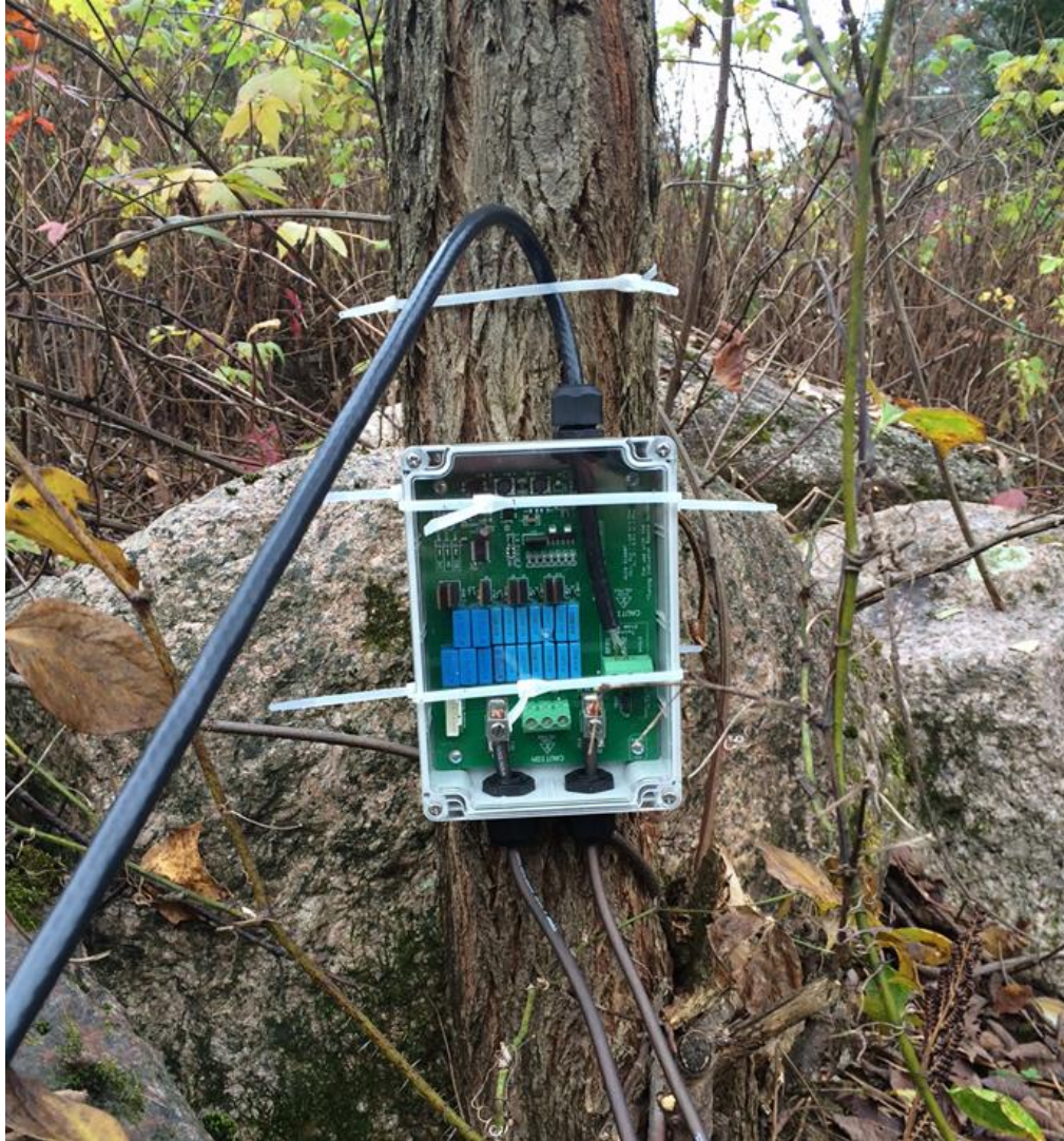
Figure 12. Oregon RFID® (Portland, OR) tuner box connected to the multi-antenna HDX reader box via Belden® 9207 twinaxial cable.
