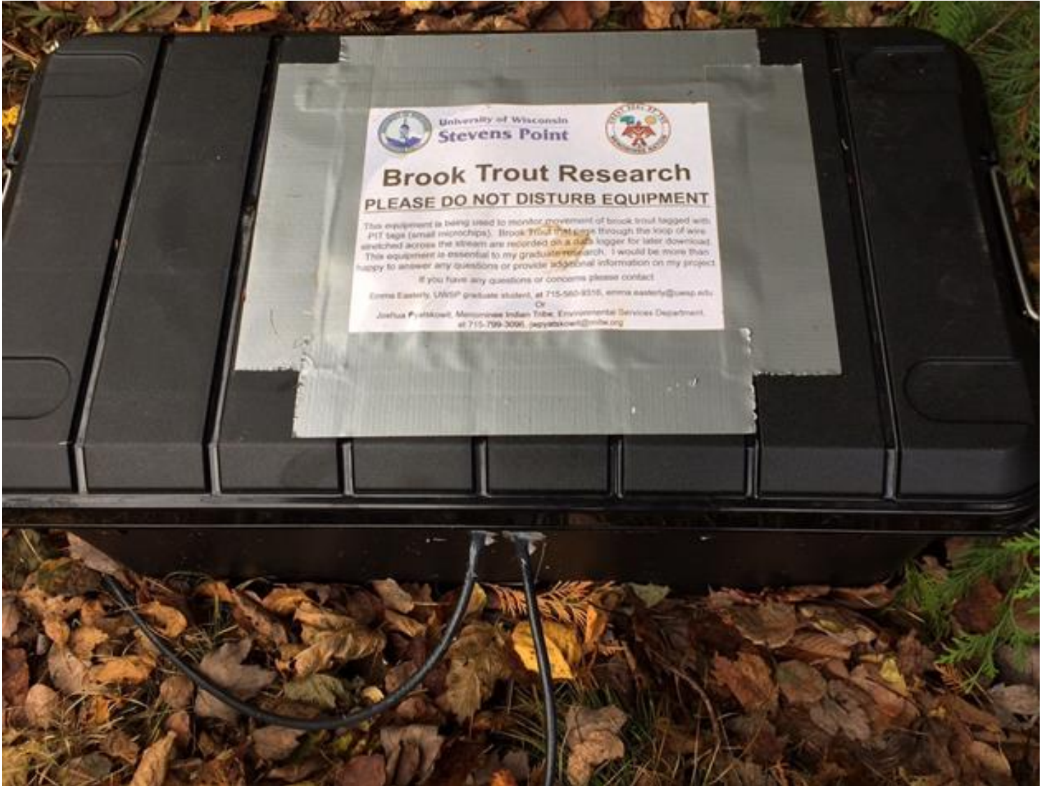
Figure 14. Plastic tote protecting Oregon RFID®, Portland, OR multi-antenna HDX reader box powered by two 12-volt deep cycle marine batteries connected in parallel.
