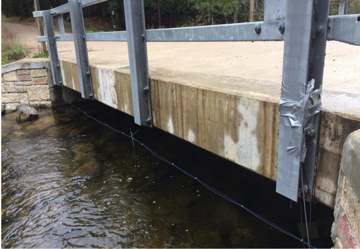
Figure 7. Upper Bass Lake antenna (1D) positioned under the bridge leading into Upper Bass Lake on the West Branch of the Wolf River, Menominee Indian Reservation, Menominee County, Wisconsin. Antenna locations are shown on the map in Figure 6.
