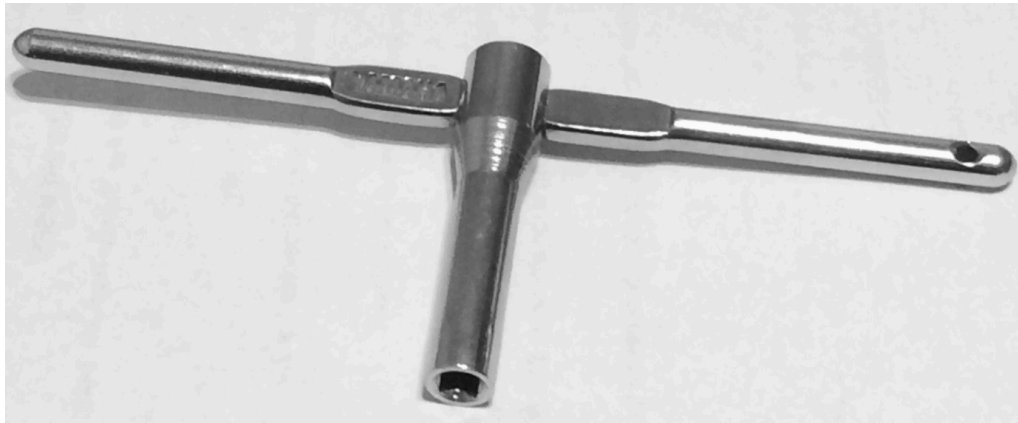
Figure 1.3: A high tension drum key or “T-key”
