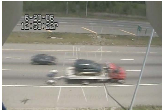
Figure 30, Examples of axle based FHWA classification errors (a) class 2 recorded as class 7, (b) class 3 recorded as class 8, (c) class 5 recorded as class 13
