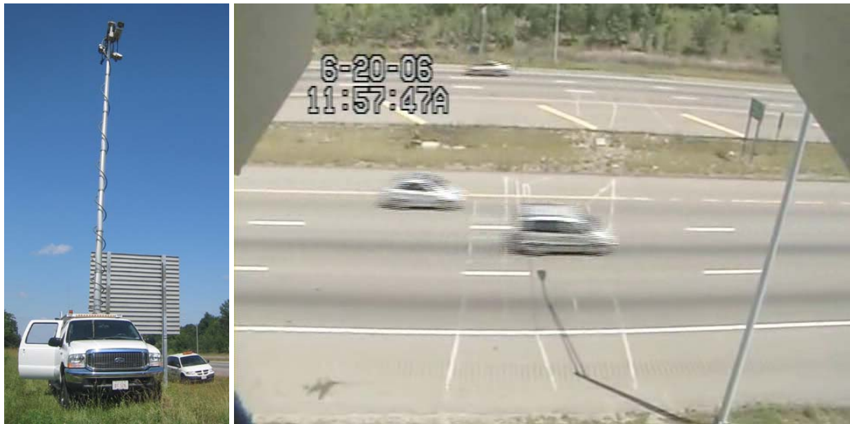
Figure 24, I70 test site, east of Brice road. The left image shows the ODOT camera truck used to monitor the detectors and the right image shows one frame from the video.
