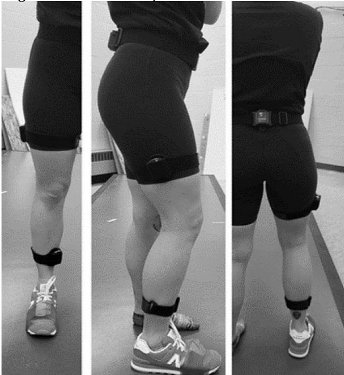
Figure 7. IMU Sensor placement
