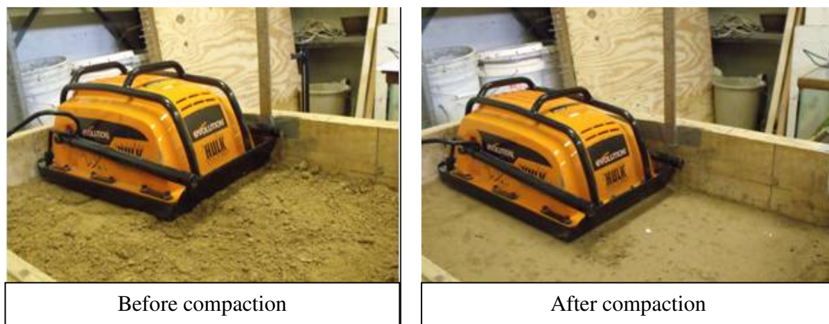
Figure 3.6: Compaction process using the compactor plate
