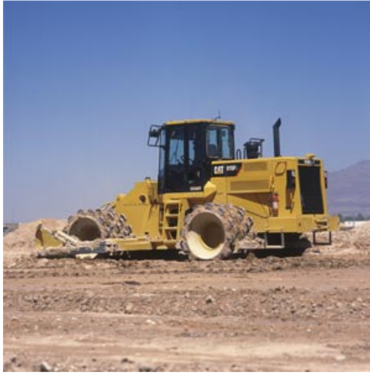
Figure 2.26: Caterpillar™ 815F padfoot roller (Operating equipment mass is 20,758 kg (45,765 lb). (Source: Caterpillar 2011))
