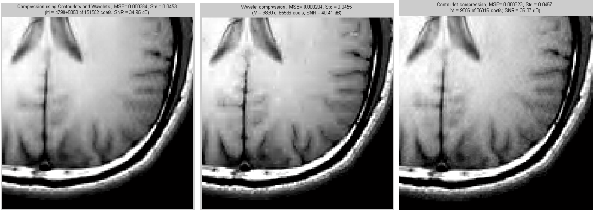
Figure 3.3: Compression keeping 15% of pixels.(from left to right) (a) Contourlet + wavelet, (b) Wavelet (c) Contourlet.
