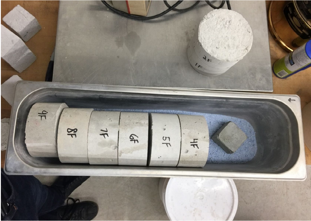
Figure 3-3: Oven-dried concrete samples being placed in a stainless-steel container to cool above Drierite™ indicator desiccant crystals.
