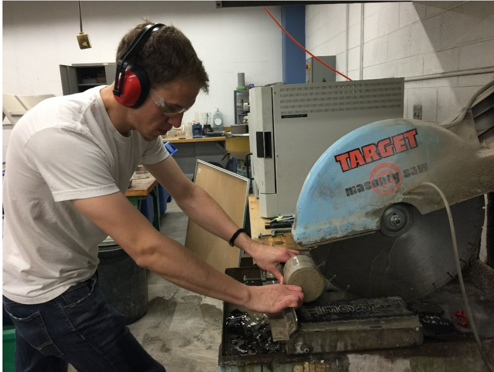
Figure 3-10: Cutting concrete cylinder samples with water-cooled diamond saw.
