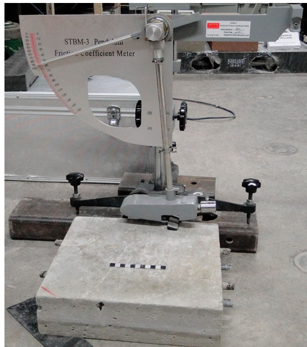
Figure 6. British Pendulum Tester and the concrete slab specimen.
