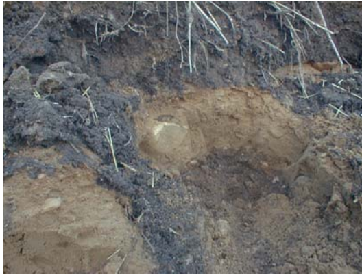
(a) Thin clay layer underlying cohesionless soil
