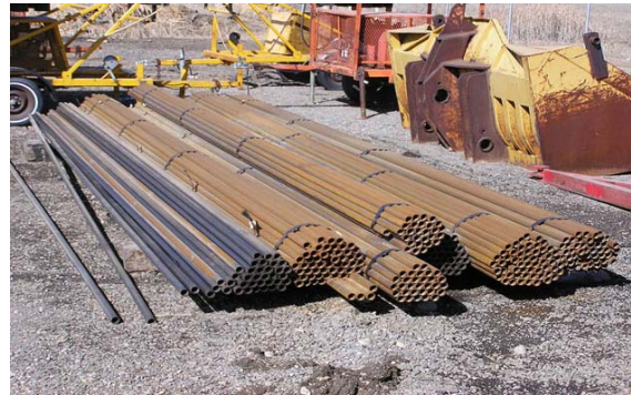
Figure 2.17: Launched soil nails of 1.5 in. diameter and 20 ft. in length (SNL, 2007).
