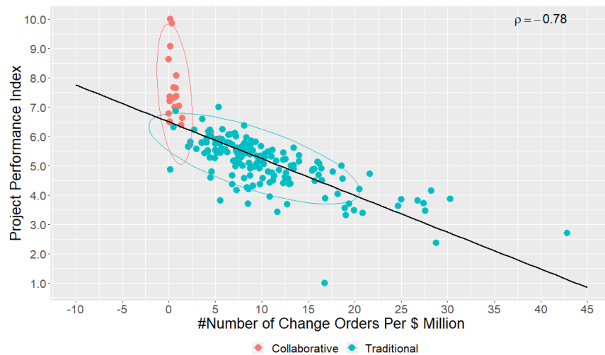
Figure 173: Plot of Project Performance Index vs Number of Change Orders Per Million Dollars
